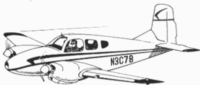
U.S. EXECUTIVE PLANE BEECH 95 TRAVEL AIR TWO 180 HP LYCOMING FLAT SIX ENGINES. FOUR PLACE. TOP SPEED - 208 MPH. CRUISE - 191/200 MPH.
