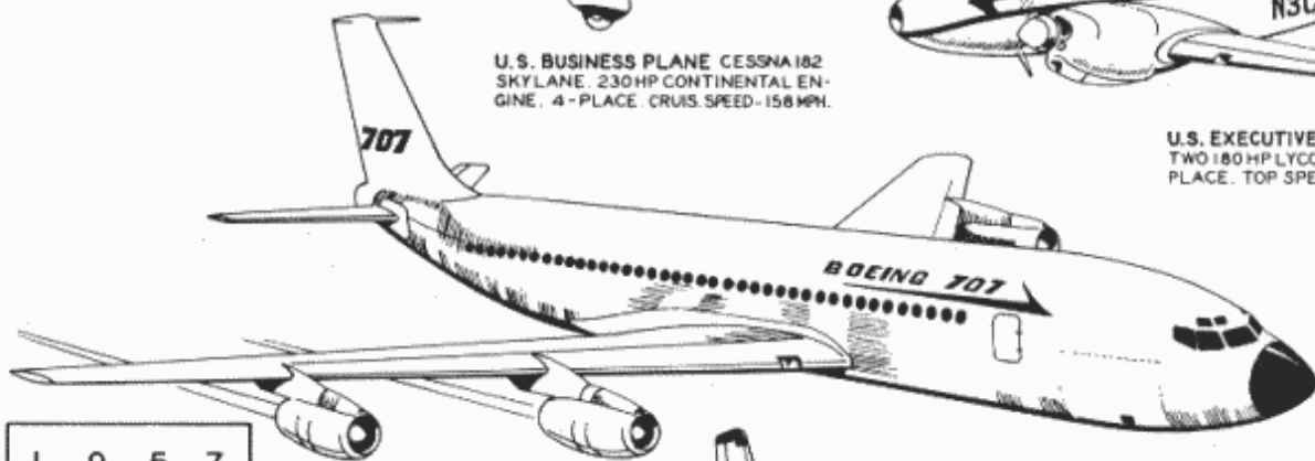
U.S. JET TRANSPORT BOEING 707 STRATOLINER FOUR PRATT & WHITNEY TURBOJETS. UP TO 180 PAS- SENGERS. OP. SPEED - OVER 600 MPH. RANGE - 5,000 M. PRODUCTION MODEL MADE FIRST FLIGHT IN DEC 57
