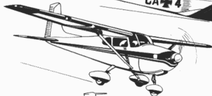
U.S. BUSINESS PLANE CESSNA 182 SKYLANE. 230 HP CONTINENTAL EN- GINE. 4-PLACE. CRUIS. SPEED - 158 MPH.
