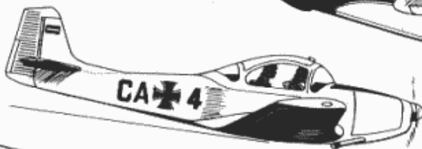
GERMAN PRIMARY TRAINER ► FOCKE-WULF P. 149 (LICENSED BY PIAGGIO) 275 HP LYCOMING ENGINE. TWO PLACE. TOP SPEED - 187 MPH
