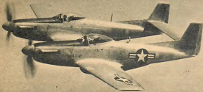
North American F-82. An all-weather fighter, it carries elaborate radar equipment capable of ferreting out the enemy despite darkness and fog. Has armament of six machine guns.
