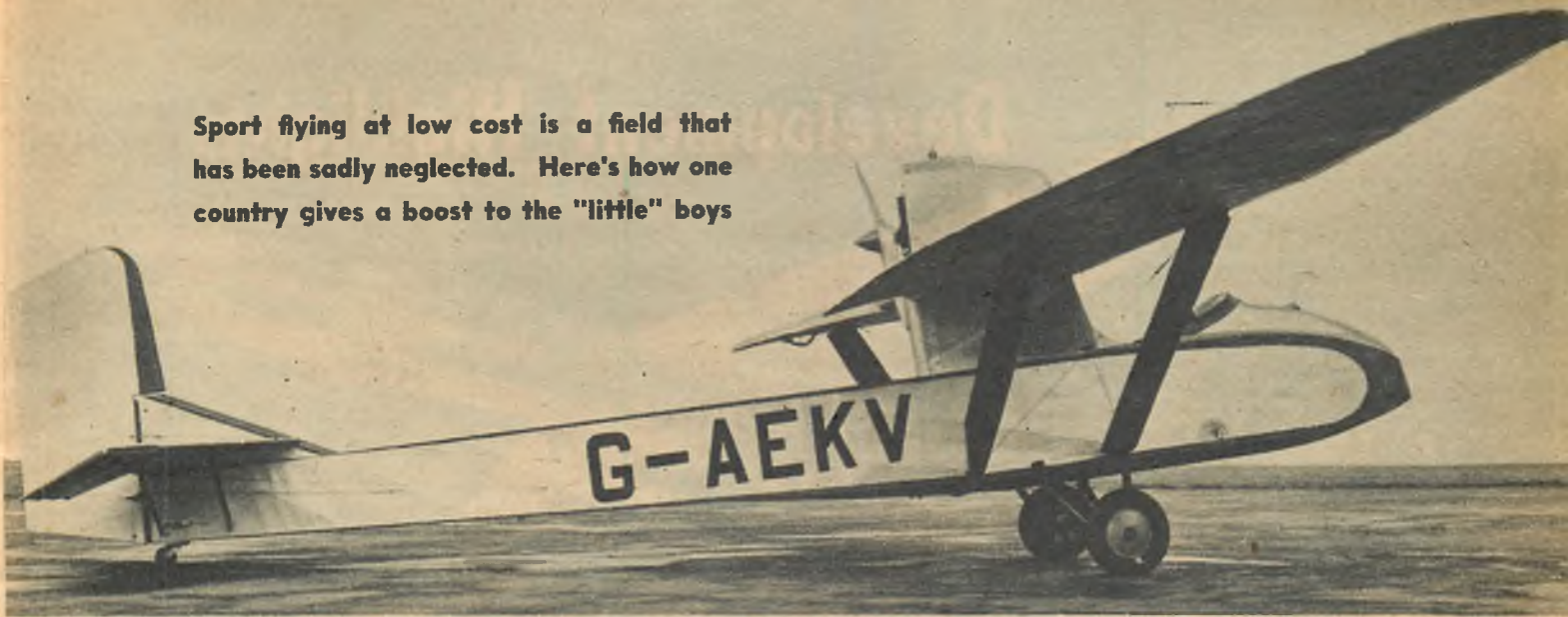
BAC Drone is actually a powered glider introduced originally by Robert Kronfeld, Austrian glider pilot. Engine is 30 hp 4-cyl. Carden.
