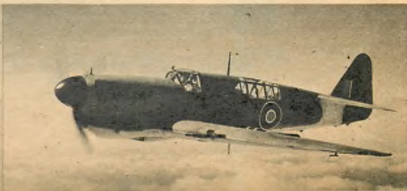
Fairey Firefly. A two-seat naval reconnaissance fighter which saw considerable service during World War II aboard British aircraft carriers. There is also a night fighter version. Plane has four 20 mm cannon.
