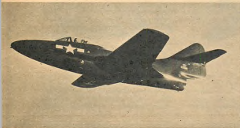
Grumman F9F. Navy's jet carrier fighter capable of speeds in neighborhood of 600 mph. Has quick take-off and slow landing characteristics due to hinged leading edge and effective flaps.
