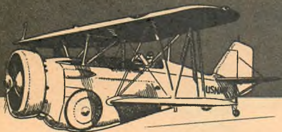
▲ CURTISS F11C-3 700 H.P. WRIGHT CYCLONE. TYPICAL 1933 NAVY FIGHTER
