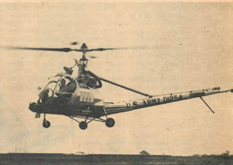
YH-23. Military version of the very popular Hiller 360 helicopter recently purchased by the Air Force for use by the Army Ground Forces. Craft also carries ambulance installation.
