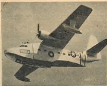
Grumman SA-16A. Latest addition to Air Rescue Service is this powerful amphibian capable of landing in high seas to effect rescue. Auxiliary wing tanks give it considerable range. Radar equipped, but unarmed.
