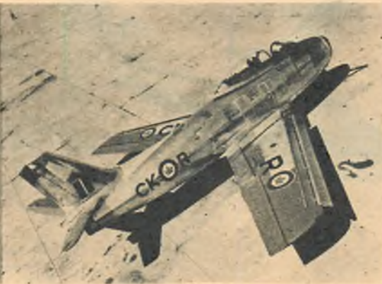
Canadian Sabre. The first of 100 Canadian-built F-86s, manufactured by Canadair Ltd. of Montreal. This model is powered by the U. S. made General Electric J-47 jet engine; subsequent aircraft will have the Canadian Avro Orenda of 7200 lbs. thrust.
