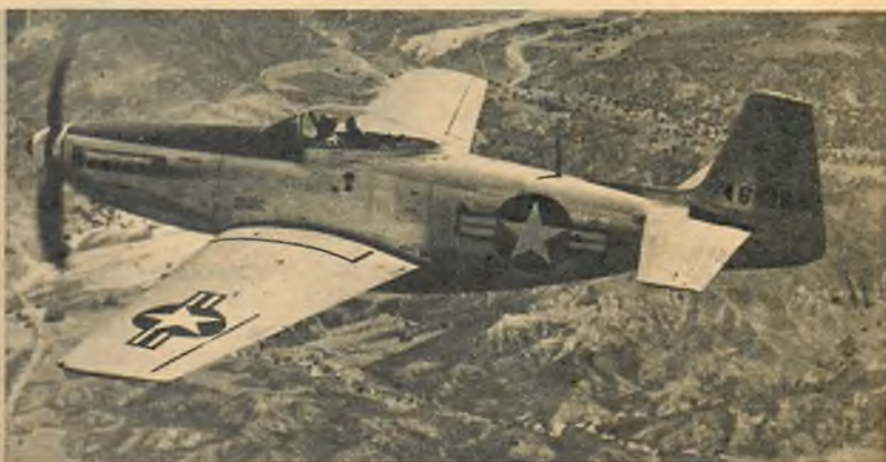
North American F-51H. Vastly improved over the original Mustang designed and built for the British in 1940. The "H" is the sixth modification powered by a 2,200 hp engine instead of 1,325 hp of the "A".
