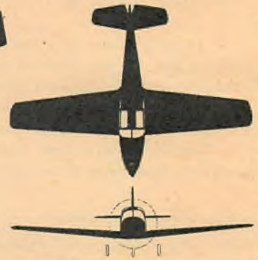
Augusta CP-110, a new Italian personal plane, is in class with early models of the Navion. Plane is of all-wood construction and powered by a 145 hp Alfa engine. Speed 170 mph.
