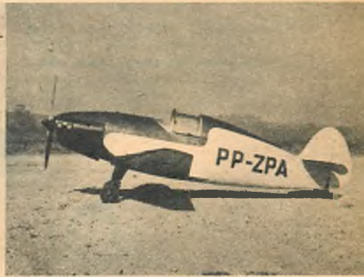
Brazilian single-place lightplane, the Bichinho I.P.T.O. designed by Institute of Technical Research to test qualities of national materials. It has a top speed of 130 mph.
