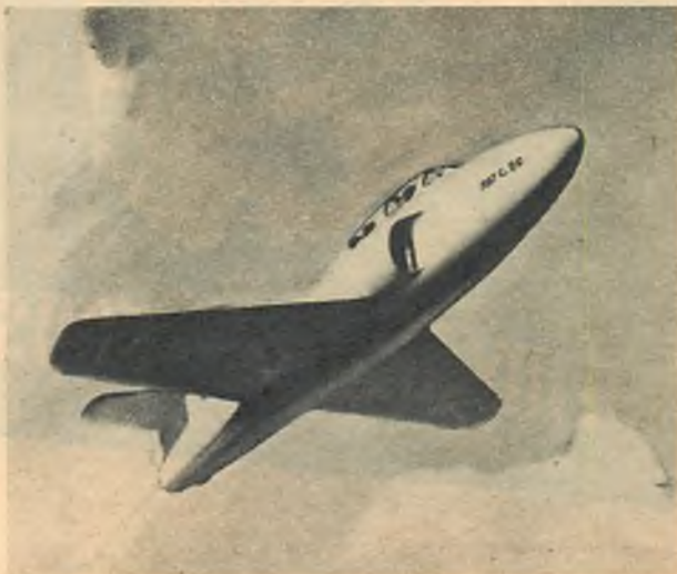
Fiat G-80. Italy's first postwar jet plane. Designed as 2-place trainer. Prototype is powered by British DeHavilland Goblin of 3500 lbs. thrust. Future models will have the more powerful R.R.Nene. Top speed 547 mph, rate of climb 5120 ft/min., gross weight totals 11,000 lbs.
