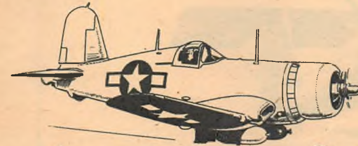
VOUGHT CORSAIR ◀ (F4U) 2,000 H.P. P. & W. DOUBLE WASP. TOP SPEED 400 M.P.H.
