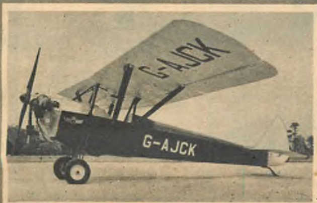
Heath Parasol. An American design quite popular here in late '20's. This British version is powered by a 36 hp JAP. Span is 31 ft.
