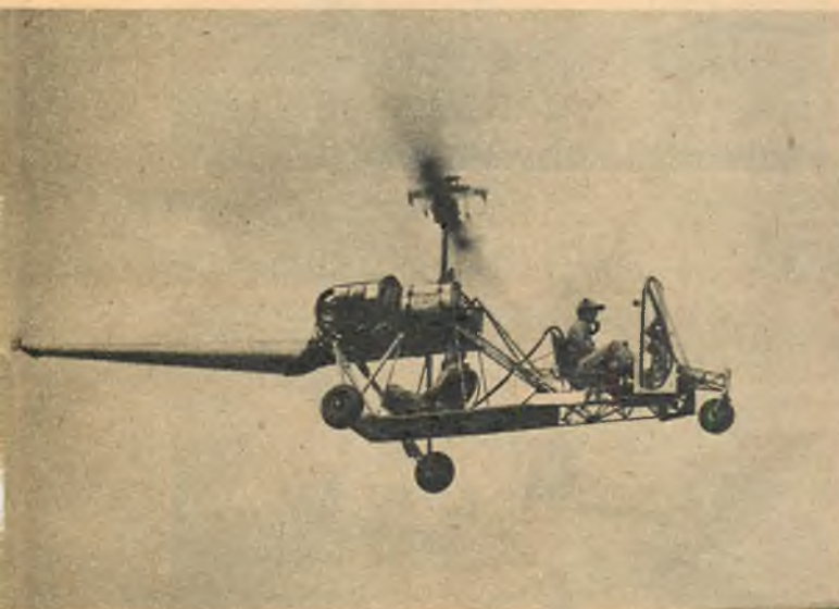
Seibel S-4 helicopter. Cargo and passenger compartment and fuel tanks located at center of lift for better balance under different load conditions. Craft's engine is a 125 hp Lycoming.
