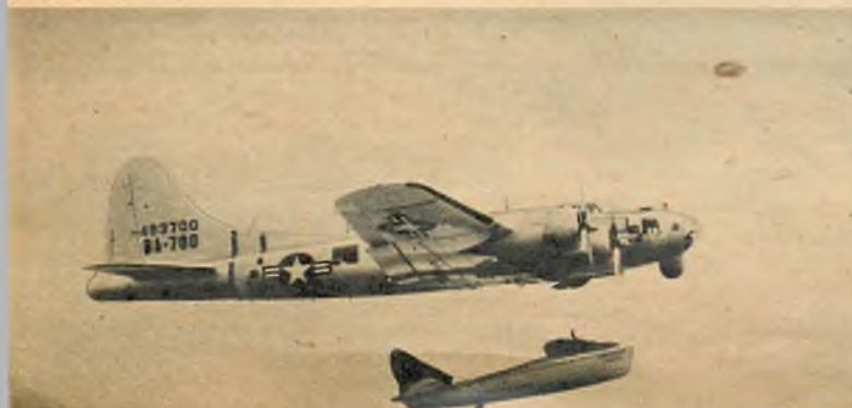
Boeing SB-17. Air Rescue Flying Fortresses were the first craft to be equipped with the air-borne boats. Because they operate in combat areas, both the SB-29s and the SB-17s are fully armed.
