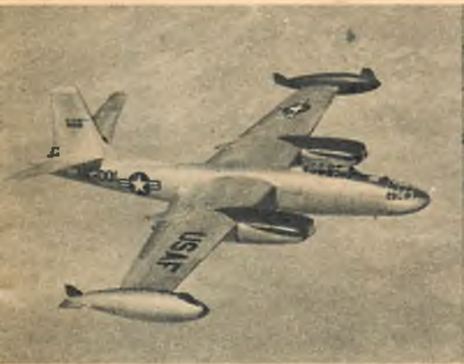
More reach is given to the North American B-45 Tornado bomber with these wing tanks whose normal range is around 800 miles. Note stabilizing fins on tanks. The pay load is over 10 tons.
