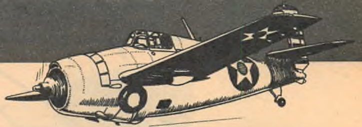
▲ GRUMMAN WILDCAT (F4F-4) 1,200 H.P. WRIGHT OR PRATT & WHITNEY EN- GINE—MAXIMUM SPEED APPROX. 325 M.P.H.
