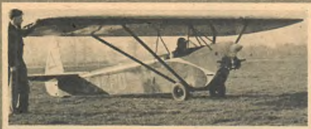
Luton Minor. Also one of the prewar oldies in ultra-lights. Span is 25 ft. Weight empty 380 lbs.; 34 hp Anzani. Top speed 75 mph.
