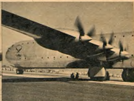
● 6 pusher engines power the craft. P & W Wasp Majors, 3,000 hp each.
