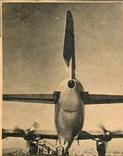
● Rear view of huge vertical fin of XC-99 soaring 57 ft. into the air.
