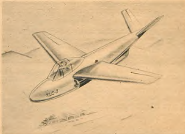
● This small single-place jet plane with wing span of only 20' 10" was designed by students of Cal-Aero Tech., Glendale, Calif. Engine is of their own design, built around type "B" supercharger. May be used as pilotless target drone.
