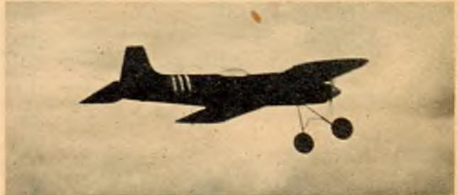
● Modified version of Tucker's Hotrock powered by Drone Diesel. Built by member of Zombie's club. Taken at annual rally of Northern Heights Flying Club held in England.
