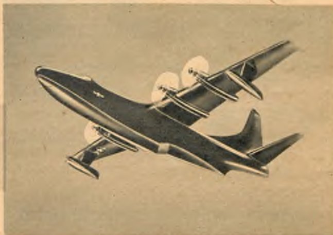
● Artist's conception of Navy's Convair XP5Y-1 patrol plane with performance comparable to land-based bombers. Two of the craft are on order. Powered by four Allison Turboprop engines. Span is 146', length 130', top speed 375 mph.
