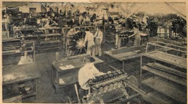
In the great engine shop at California Flyers the mechanic trainee assembles, disassembles and repairs every type of aircraft engine.
