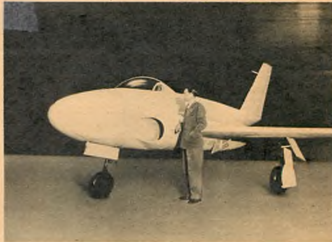
● Mock-up of latest entrant in the field of sonic speed, the Northrop X-4, now undergoing tests at Muroc Air Base. Features low-drag flying wing principle. Powered by 2 Westinghouse J-34 jets, 3,000 lbs. thrust each. Span 25'.
