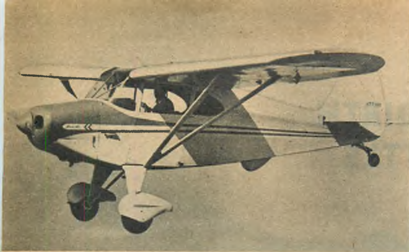
1951 Pacer , built by Piper Aircraft Corp., is offered this year in two models, both powered by 125 hp Lycoming. The 135 is equipped with a controllable prop while the 125 is not. Both models have flaps. Both finished with a plastic non-flammable covering. Span is 29.3'.
