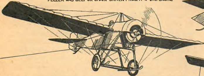
1912 BLACKBURN WAS CLEANER, MORE POWERFUL. ▲ THAN 1911 MODEL. RECENTLY THIS PLANE WAS RECONDITIONED AND FLOWN WITH THE ORIGINAL 50-H.P. MOTOR
