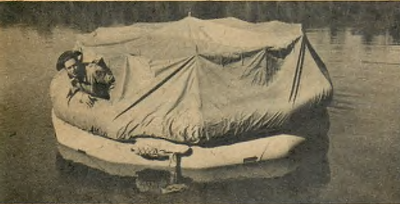
The floating tent above is a 20-man life raft developed by Air Materiel Command for use in ditching operations. With its canopy and sides up it is snug and dry as well as highly buoyant. The canopy has a radar reflector to facilitate search.
