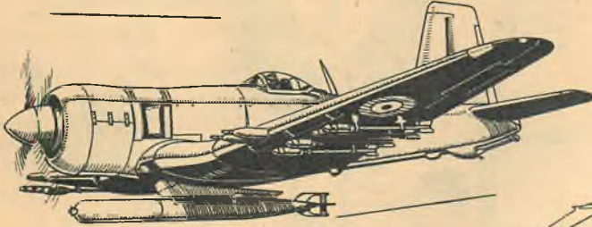
▲ BLACKBURN FIREBRAND V. STANDARD BRITISH NAVY STRIKE FIGHTER TODAY. THIS 2,500-H.P. HEAVILY ARMED PLANE IS ONE OF WORLD'S TOP PISTON-ENGINE DESIGNS BUT IS ALREADY DATED BY THE FASTER JETS
