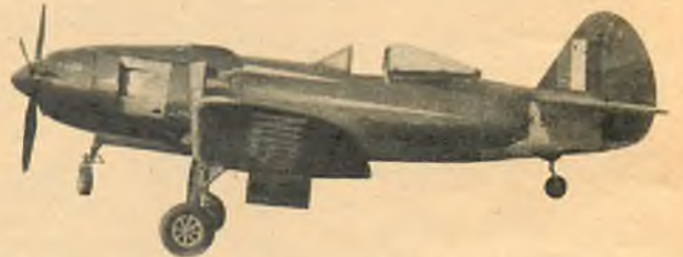
This mighty fighter even sports a small nose wheel just in case the long nose has a tendency to do some ground plowing on landing. Front, Curtiss XF15C; middle, Corsair FG-1; tail section, Curtiss P-40.
