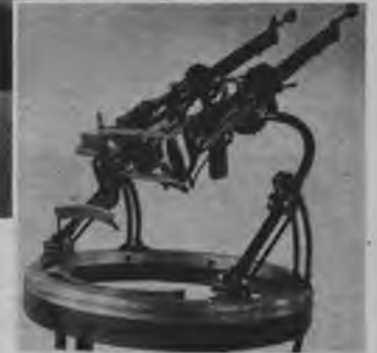
Familiar to old-time combat pilots was the Scarff mount for twin Lewis guns.
