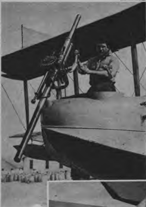
1920: Combination machine gun and Davis cannon was tested on navy flying boat.
