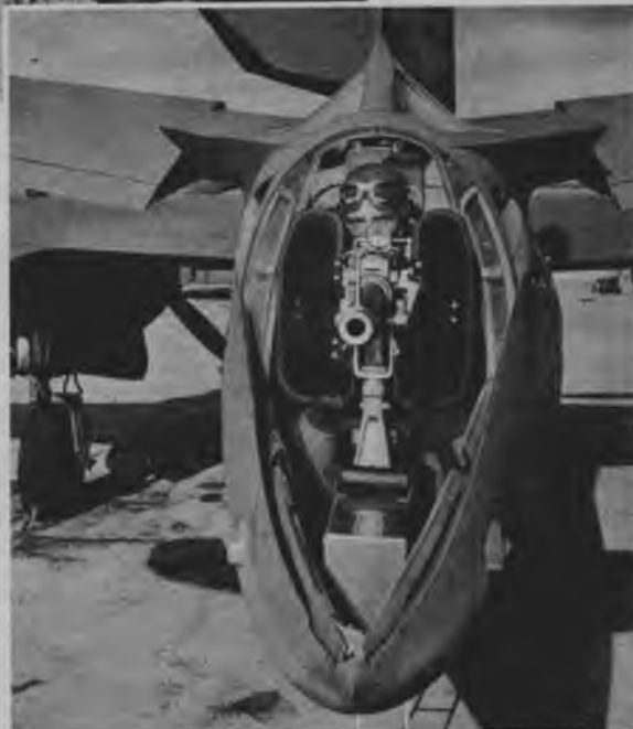
The powerful .50-cal. tail gun in a Martin B-26 typifies the modern armament on aircraft. Bigger and better guns are on the way.
