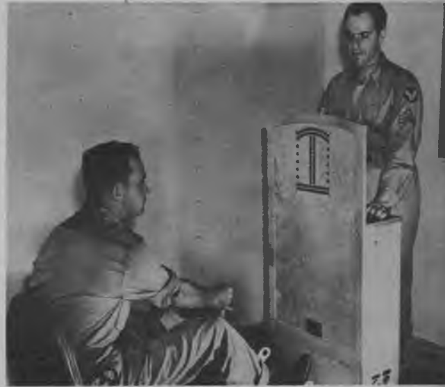
Feet on rudder bar and hand on stick, cadet tries to bring red and green lights on reaction board into straight lines.
