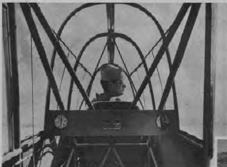
Student in the front seat of an Aerona TG-5 three-place glider. Note large "greenhouse" allowing exceptionally fine visibility.
