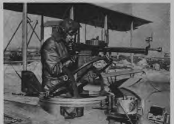
Single guns were also mounted on Scarff ring-mounts. Yoke raised and lowered and entire mount swung in circle. Gunners were ho-men.
