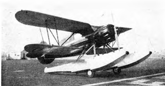
Waco CUC amphibian is powered with 250 h.p. Wright Whirlwind engine. Floats are of Edo design with retracting wheels. Ship can be quickly converted to conventional landplane.
