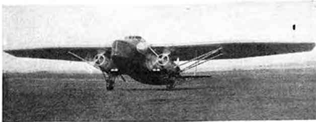
Giant 44-passenger Farman airliner is powered by 4 Knome Rhone 800 h.p. engines. Span is 118 feet.
