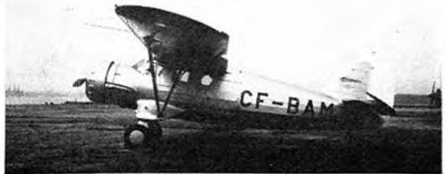
Latest Norseman design built by Noorduyn Aircraft, Ltd., of Canada, 450 h.p. Wasp motor, has the usual Noorduyn landing-gear projections which support floats when attached.
