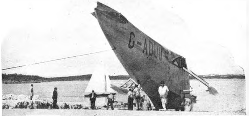
Hull of the 18-ton British flying boat "Cavalier," being drawn up on the beach at Bermuda preparatory to assembly. The "Cavalier" is one of a number of flying boats intended for trans-Atlantic service in the spring.
