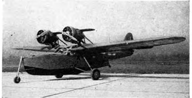
The army's new nose-wheel amphibian is an experimental version of the Douglas Dolphin. The engines are Pratt & Whitney 450 h.p. Wasps. Note the position of the ship as it rests on all three wheels.
