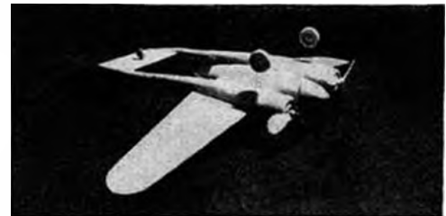
Here the unpainted G-1 is shown inverted. Note the installation of the tail wheel and landing gear.
