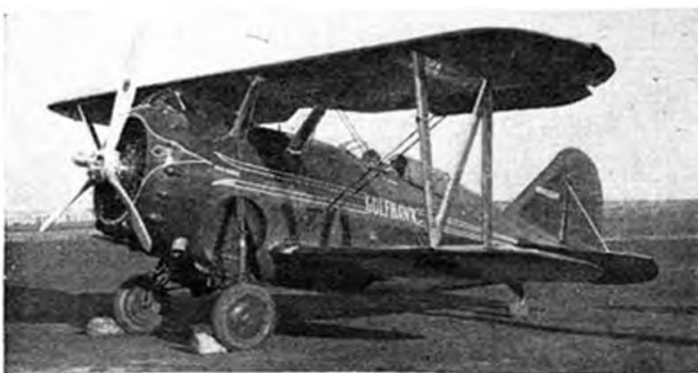
Al Williams' Gullhawk, a Grumman G-22, is similar to the navy's F3F-1. Power plant is the 935 h.p. Wright Cyclone.
