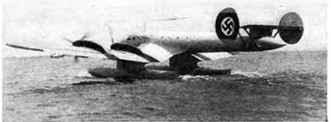
The 4-engined Hamburger Flugzeugbau Ha-139 has been developed for the Deutsche Lufthansa. Despite its size, launching is to be done by catapult. This plane will be placed in the German transatlantic service to America.
