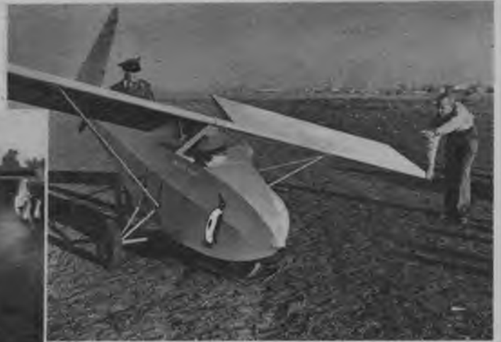
Before being towed, the student is taught to keep the wings level; improper control may otherwise cause the trainer to damage wing tips.
