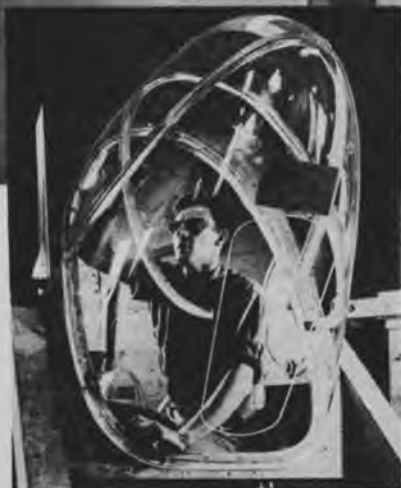
Something to consider. This bomber nose made by Du Pont is entirely of Lucite, including ribs.
