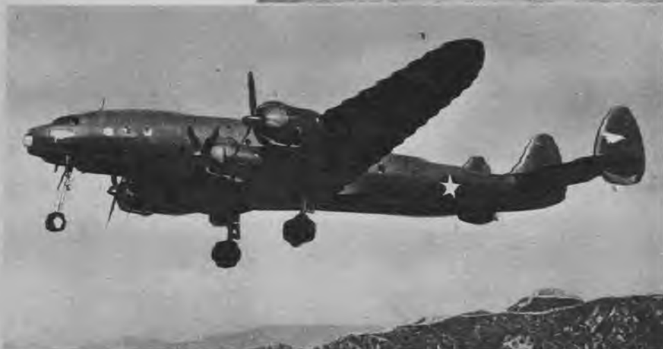
Lockheed Constellation, new giant cargo plane, takes to the air on its maiden flight. Powered by four 2,000 h. p. engines, it has pressurized cabin for flying at 35,000 feet, can cross the continent in 9 hours. Flying at cruising speed.
