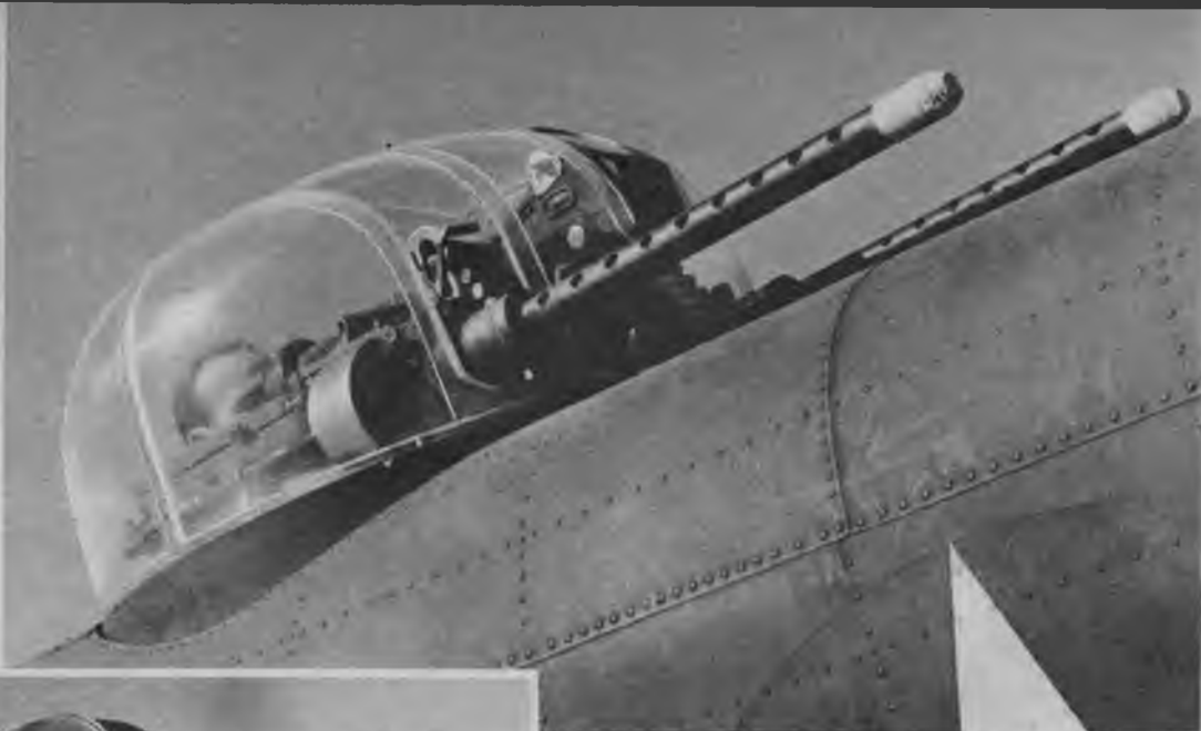
Half-hidden gunner in Martin turret sights in special eyepiece. Muzzles of guns are taped to keep out dirt, moisture, prevent rust.
