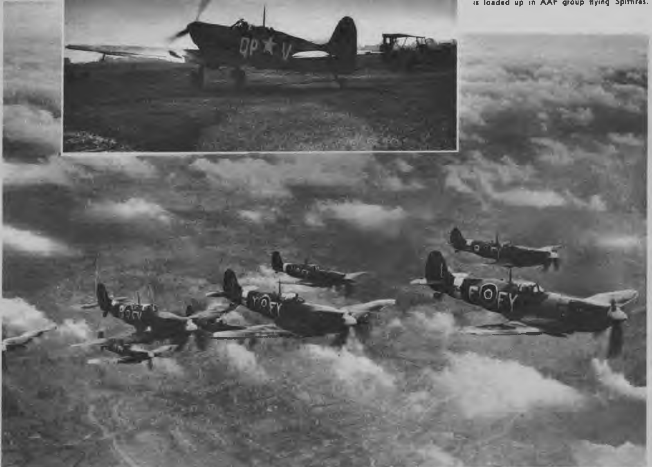
High above the clouds is a squadron of the latest high-altitude Spitfires. Four-bladed propellers and highly supercharged engines permit fighting at extreme altitudes.
