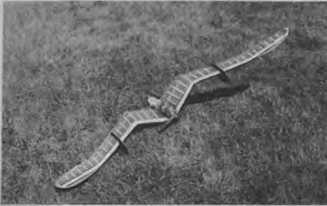
The rubber version of this design produced flights of over a minute and a half. It proved slightly tricky as a gas job; the wings were found too weak.
