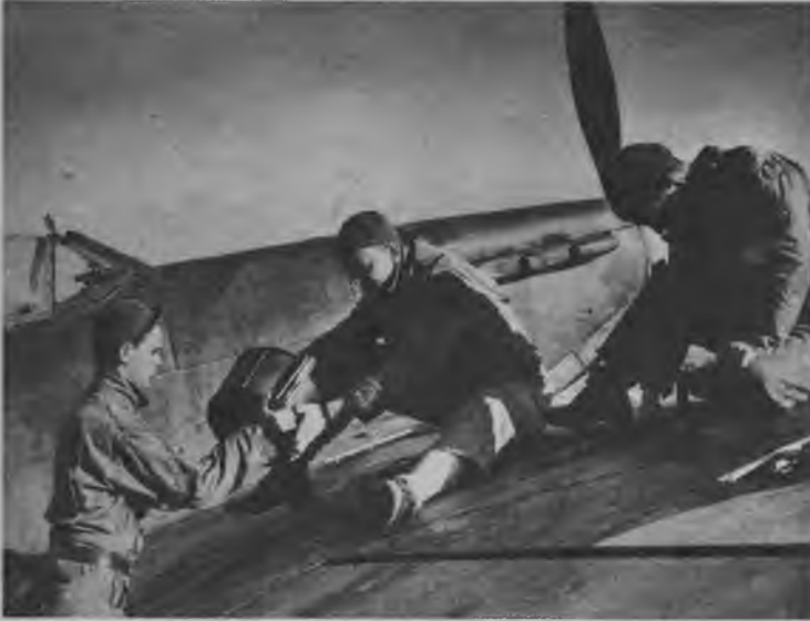
Drum containing shells for one of the two 22-mm. Spitfire cannons is placed in wing by armorers.
