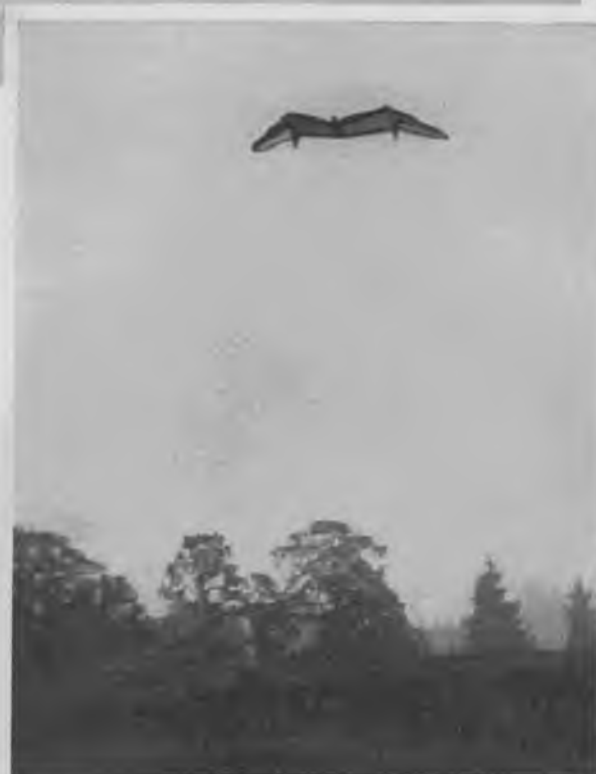
Design No. 3 was lifted directly from bird study. It features flexible slotted tip ailerons, uses airfoil developed exclusively for flying wings.
