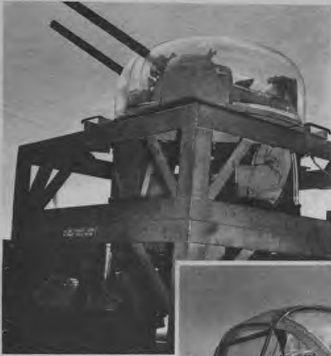
As student elevates guns of the truck-mounted Martin turret, the mechanism automatically swings him lower to keep target in his sights at all times.
