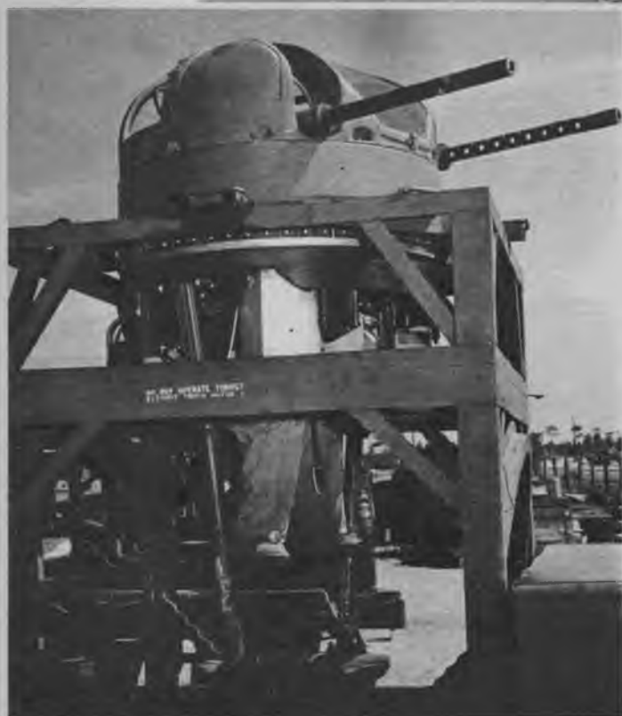
In Sperry Fortress turrets mounted on moving trucks gunners learn to "lead" enemy planes. Turrets are operated by electric or hydraulic power. Some have armor plate.
