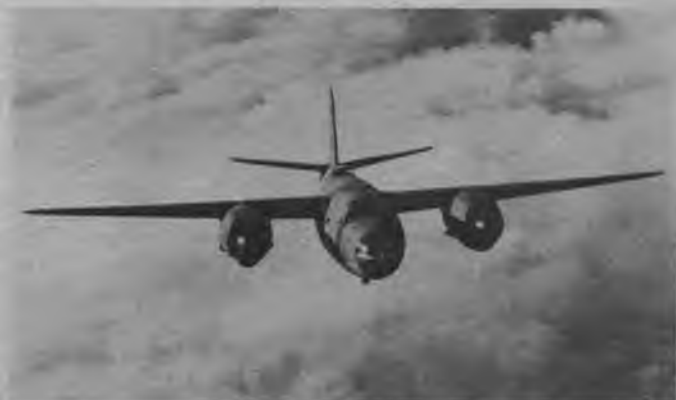
The Martin B-26 Marauder, two 1,750 h. p. engines, presents about the cleanest lines of any aircraft. This fastest medium bomber has top, nose and tail turrets.
