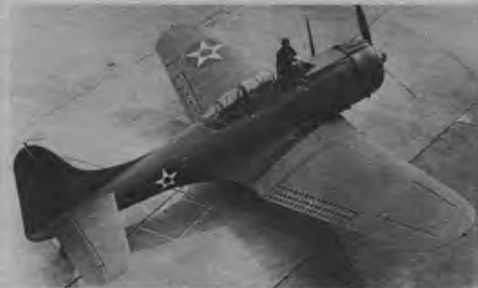
The Douglas A-24, is the army dive-bomber version of the navy's Douglas SBD-1 scout bomber. The split perforated flaps prevent tail buffeting in dives.
