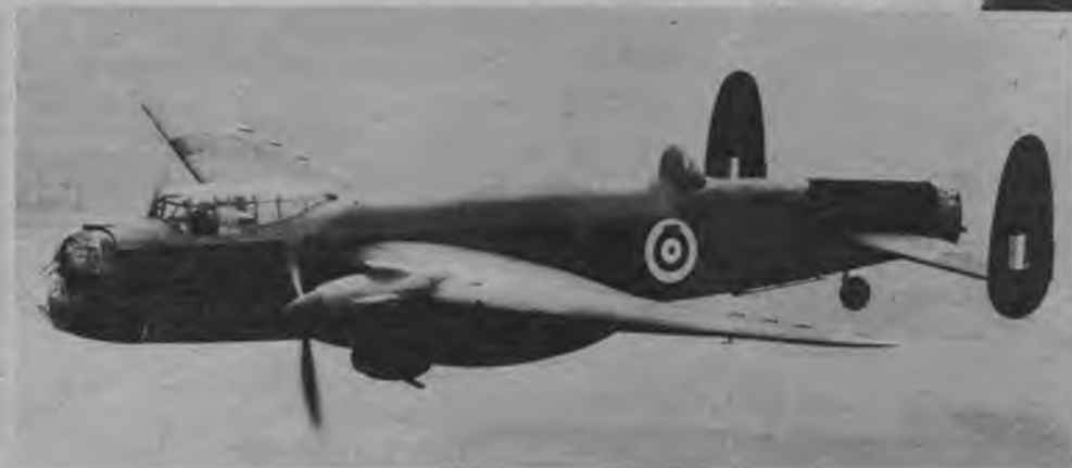
The new Avro-Manchester bomber, though having only two engines, is one of the most powerful. The two Rolls-Royce Vultures of 2,000 h. p. each give this long-range bomber exceptional performance. Note top, tail and nose turrets.
