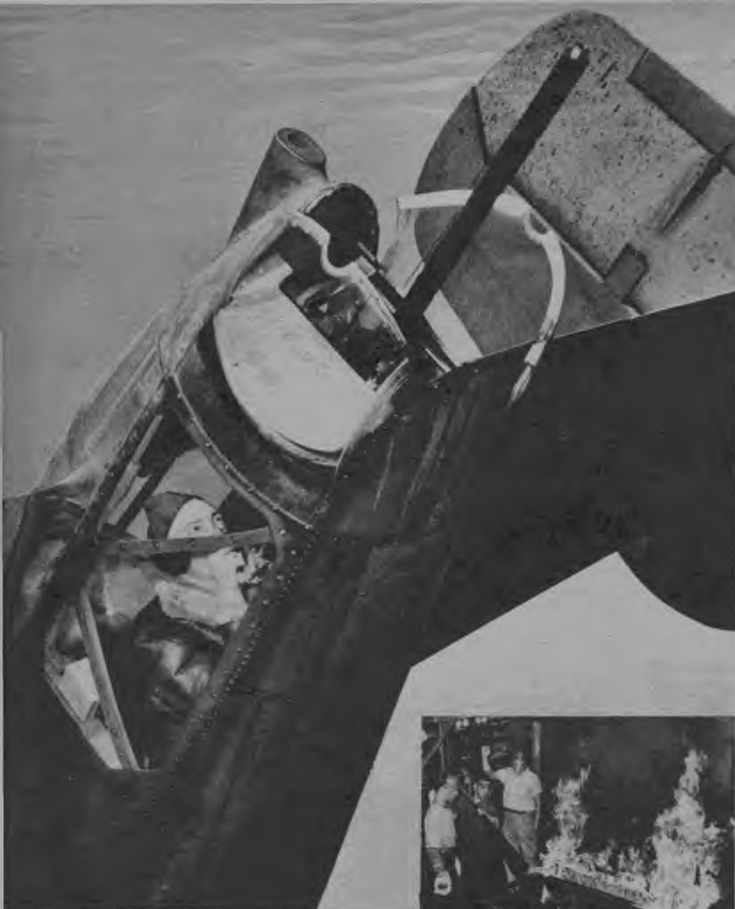
Protection for the stinger. This released photo shows the deflecting armor plate in tail turret of N. A. B-25.
