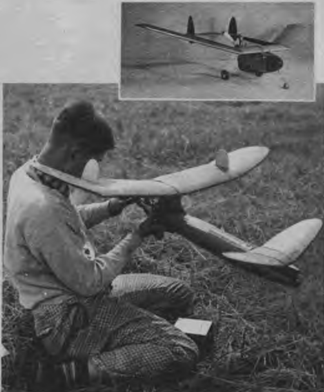
Above—Pixie. Center-of-gravity problem is solved by highly swept-back wings. Below—Pusher plane. Standard canard setup. Model flew at '41 national contest.
