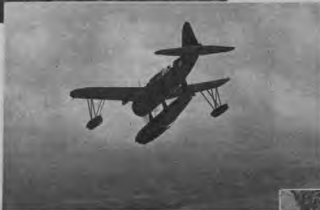
Vought-Sikorsky Kingfisher used by cadets of the Jacksonville Naval Air Station for dive-bombing practice. Top picture shows ship on the way to target. Below: Approaching target, the ship is put in diving attitude which is gradually steepened until (right) the target is lined up in bombsight and the fifty-pound practice bombs are all released.
