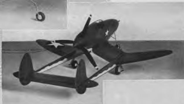
This semiscale job is a real prop saver because of pusher arrangement with tricycle landing gear. Note detail of guns and exhaust.
