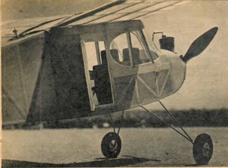
● Clean lines of Kothe's 1st-place winner evident here. Door must be wide enough to admit "passengers," weighing 8 ounces each.
