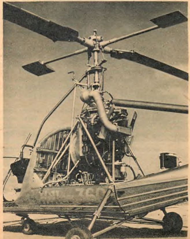
● Short rotor blades are servo-tabs that control rotor pitch. Note simple control linkage. Rear pipe is carburetor air intake.
