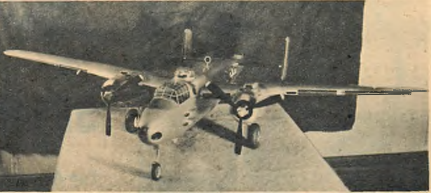
● Super-detailed non-flying scale B-25, work of Paul Nock, Albany, N. Y. Took over 1,500 hours. He used 1/16" sheet balsa with 15 coats of filler and dope. Motors are built up and incorporate all external parts of prototype. 75-mm cannon in nose, Plexiglas turret, shock-absorbing gear.
