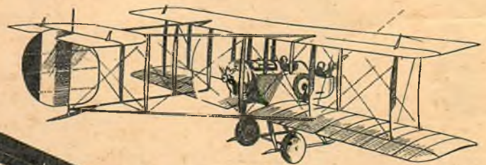
1914-15 VICKER "GUN BUS" 100-H.P. MONO-Gnome (A VERY EARLY APPROACH TO THE PRESENT-DAY ATTACK PLANE.)
