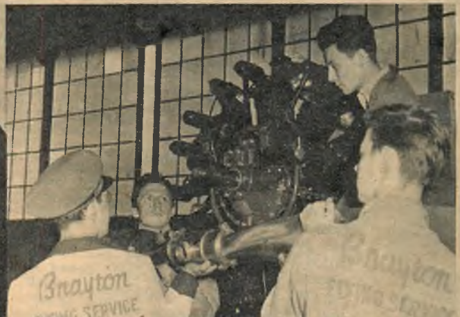
● Students practicing propeller installation. In the engine mechanic's course they are given practical training on variety of engines.
