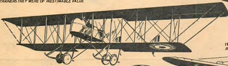
1914 MAURICE FARMAN "LONGHORN" (ABOVE) AND "SHORTHORN" (BELOW). BOTH POWERED WITH 70-H.P. VEE-8 AIR-COOLED RENAULT ENGINES. THEY HAD NO ARMAMENT AND SOON PROVED MUCH TOO SLOW FOR PRACTICAL MILITARY PURPOSES BUT AS BASIC TRAINERS THEY WERE OF INESTIMABLE VALUE.
