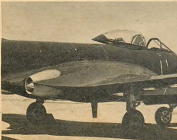
● Close up of wing root and jet engine shows how nicely power plants have been arranged. Wings fold for storage aboard carrier.
