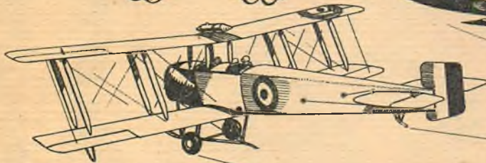
1914 AVRO 504-K 80-H.P. Gnome ROTARY. EMPLOYED AT FIRST AS AN ALL-PURPOSE WARPLANE IT WAS SOON WITHDRAWN FROM ACTIVE SERVICE TO BECOME, IN MODIFIED FORM, THE TOP BASIC TRAINER PRODUCED DURING WORLD WAR ONE.
