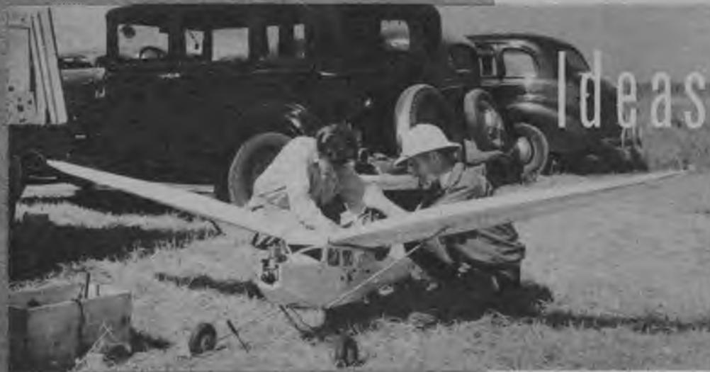
Beauty of radio control is realism of the model in the air. This job is built like a real ship, has hardwood longerons, plywood nose covering, is assembled with screws and nails.
