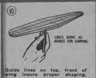
Guide lines on top, front of wing insure proper shaping.
