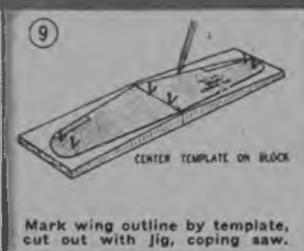
Mark wing outline by template, cut out with jig, coping saw.
