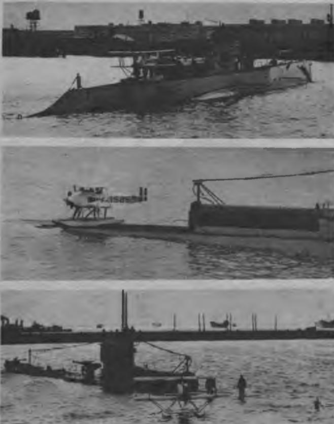
Not so many years after the close of the first World War there appeared the first plane-carrying submarine, the U. S. S. S-1. This tiny Martin seaplane was assembled on deck and launched by submerging rear of submarine.
