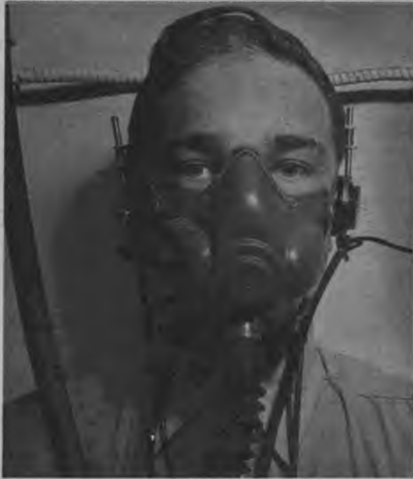
In the old days pilot "sucked" on tube for oxygen; today's mask incorporates reservoir, effects 75% saving, warms, humidifies oxygen.
