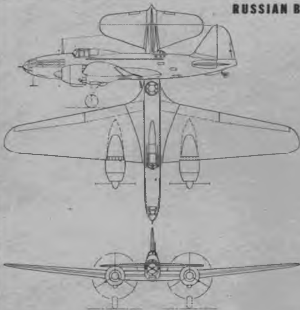
DB-3F. A fairly fast, clean-looking job, this ship is about the size of our Douglas DC-3 airliner. Its 1,000 h. p. M-88 engines are neatly streamlined in small-diameter cowlings. Lifts big load.
