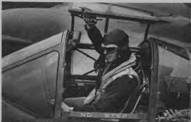
Lightning rider. Thick bullet-proof glass inside windscreen; radio behind cockpit; oxygen bottle, right foreground; inflatable life belt around pilot's neck.
