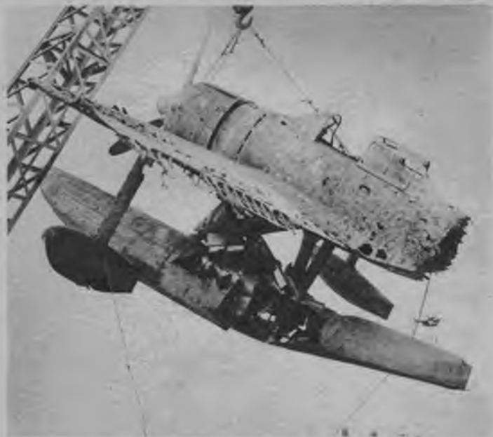
Seaplane Zero has unsurpassed cleanness for a floatplane, though it looks flimsy. Among tricks are fuel tank in the pontoon and oil-cooling radiator in main strut.
