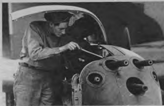
Since synchronization is not required guns shoot at maximum rate of fire. All-in nose, they are: two .50 caliber; two .30 caliber, one 20 mm.
