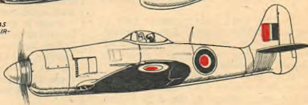
HAWKER FURY LAST OF A LONG LINE OF PISTON ENGINE HAWKER FIGHTERS (1914-49); TOP SPEED WITH 2,025-H.P. ENGINE EXCEEDS 450 M.P.H.
