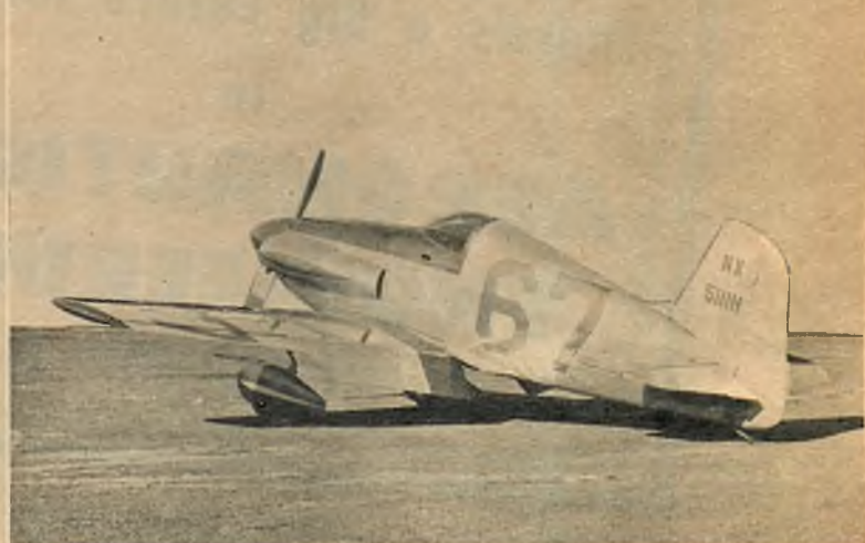
● For the sportsman. Midget Mustang, designed by David Long of Piper Aircraft, and flown by him in races at Cleveland and Miami. Ship is very easy to fly, has cruising speed of 170 mph. Will be produced commercially by Schweizer Aircraft Corp., Elmira, N. Y.
