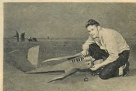
• Now this is what you can call a really different ship! Tommy Counter, Los Angeles, built it. The V-tail biplane is powered by g.p. Ohlsson .60.
