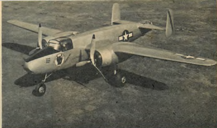
• "The Snorting Bull" is 55" scale B-25 powered by two K&B Torpedoes. Does about 75 mph. Built by Harry O. Porter, Jr., Birmingham, Ala., from modified Cleveland kit. From insignia, the prototype flew 14 missions, sank three Jap warships. Model looks fully planked. Note pilot in front office.
