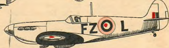
VICKERS SUPERMARINE SPITFIRE* 1030-H.P. ROLLS-ROYCE MERLIN. TOP SPEED 367 M.P.H. - 8 GUNS -
