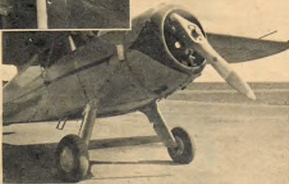
● Photo A—single-bladed propeller on Cessna Airmaster. The single-blader was first successful automatic v.-p. prop.
