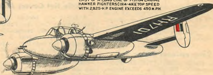
BRISTOL BRIGAND STANDARD LONG-RANGE ATTACK BOMBER AND NIGHT FIGHTER. MOST RECENT DEVELOPMENT OF THE BASIC BLENHEIM DESIGN.
