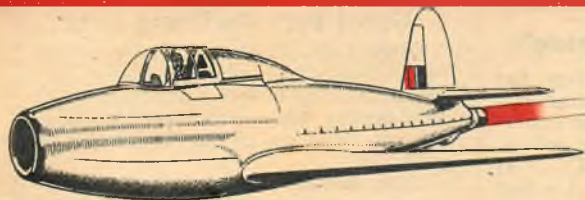
GLOSTER E28-39 ORIGINALLY DESIGNED AS A FLYING TEST BED FOR BRITISH TURBO-JET ENGINES.
