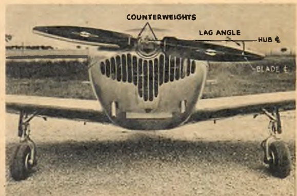
● Photo B—Swift equipped with Aeromatic prop. Note lag angle formed by hub's center line and center line of blades.
