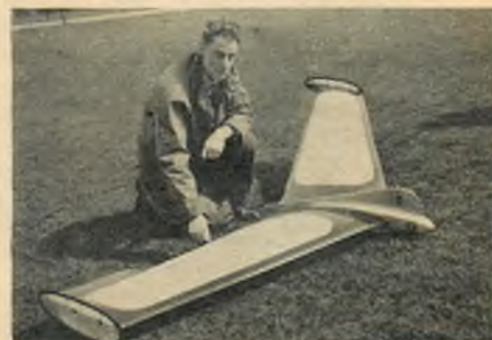
• Tailless sailplane of 8 1/2' span made by A. J. Cockle of Northampton (England) MAC. RAF 32 wing section; weight 5 1/2 lbs.; movable elevons.
