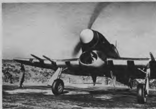
Huge air scoop houses engine air intake, cooling for both oil and liquid radiators. Four long-barreled 20-mm. guns may be high velocity.
