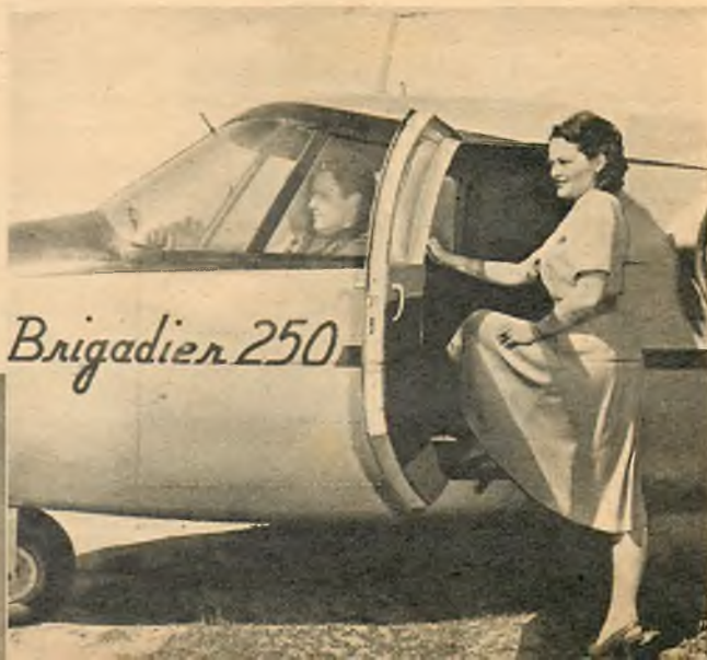
● Getting into cabin is like stepping into a car. Step is 20 inches above ground. No danger from propeller or slipstream.
