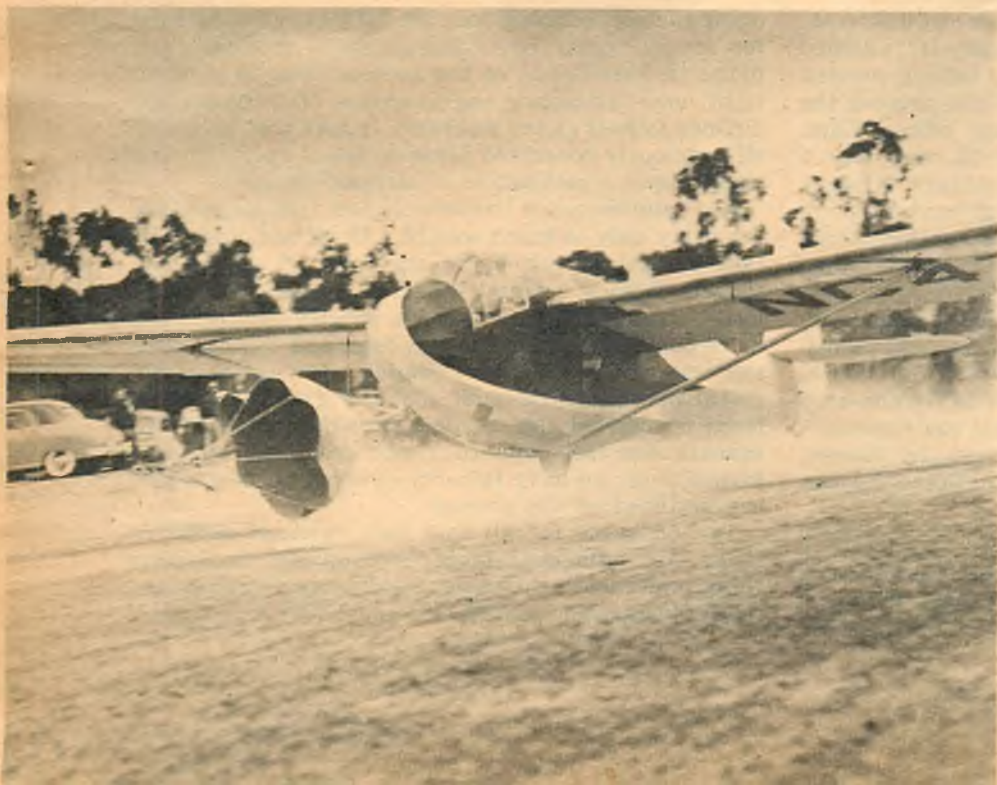
● Winch take-off by Dick Johnson in Schweizer. Chute keeps wire straight after release.
