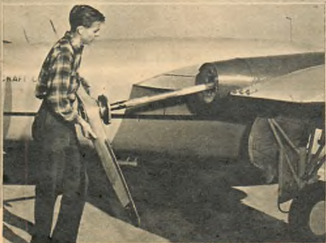
● Pusher propeller shaft slips out by unfastening three bolts. It is secured on a floating mount which absorbs vibration.
