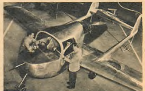
Northrop student engineers consult on dual control arrangement for student-designed and built private plane. Complete metal mock-up shown here was fabricated and assembled by students as part of practical training project.
