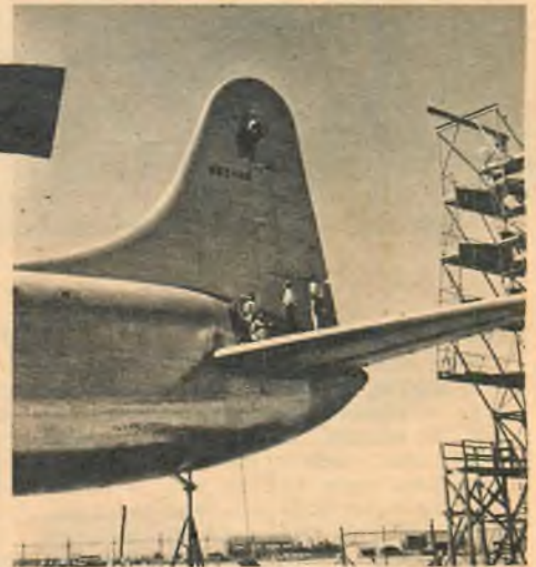
BIG JOB for engineers was inspection of completed 57-foot-high tail fin on Air Force's XC-99 Consolidated Vultee transport, world's largest land plane... an example of the interesting and varied duties performed by aeronautical engineers.
