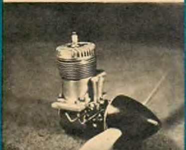
● Ervin Napravnik, Czech engineer, made this .64 engine. Horsepower, .8; wt., 14 oz.; maximum rpm, 13,600.
