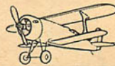
Laird Super Solution biplane for U-control. Has span of 26 inches. Takes Class A engine. Part of Plan 103.
