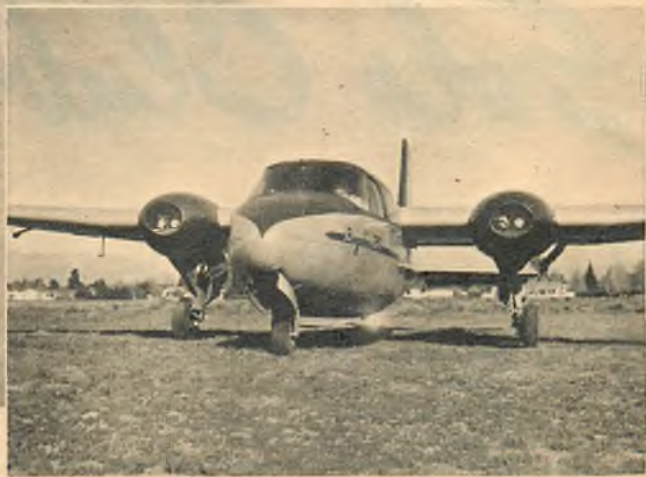
● Tricycle landing gear permits a level, automobile-height cabin. Slanting nose gives good visibility while taxiing on the ground.
