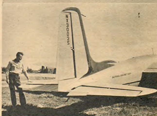
● All tail surfaces of the Brigadier are identical. This greatly simplifies production and makes replacement an easy matter.
