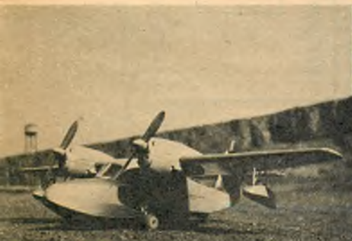
• Rubber job revamped into 50 in. gas model: AT's Grumman Widgeon 2 Forster 29's by Hans Messmer, N. J.
