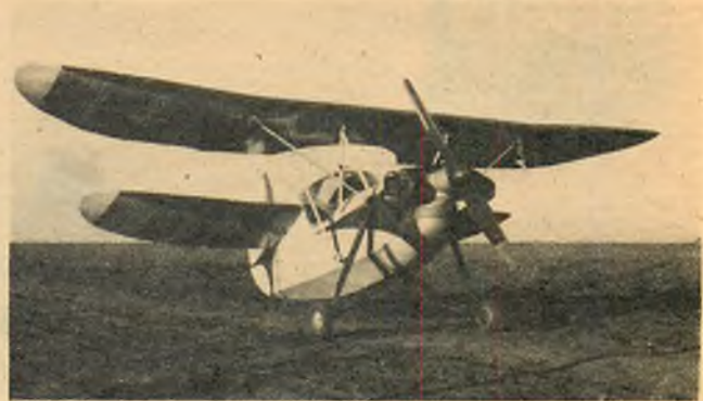
● The Mignet H.M. 294, rechristened Butterfly, was built in Argentina. This single-place machine is powered by a 35 hp Aeronca.
