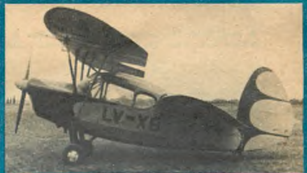
● H.M. 300. Clearly shown is extremely short moment arm.
