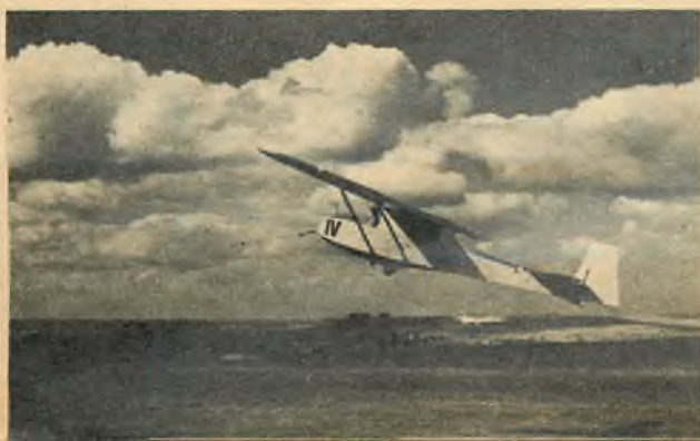
● Slingsby Tutor launched by winch. This method is used for the advanced student. It requires much more alertness than auto-tow.
