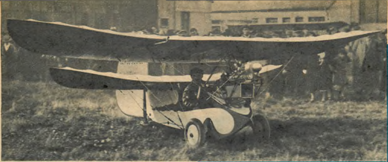
● First of the Flying Fleas, the H.M. 14 at Orly, France, in 1935. Engine is a 2-cycle, 2 cylinder, Aubier & Dunne, developing 17 hp.
