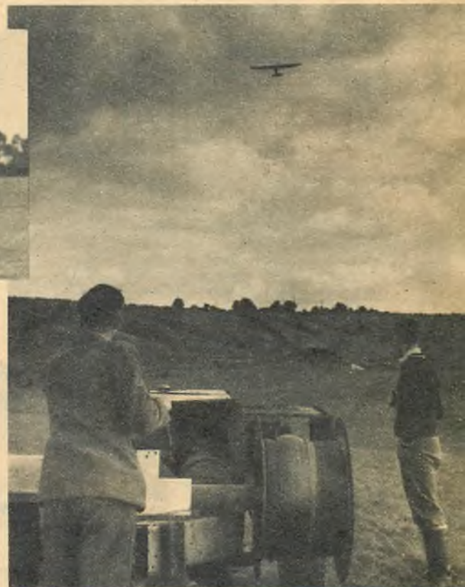
● Cheaper than U.S. aero-tow method is that of launching by a winch. Auto-tow is also used.
