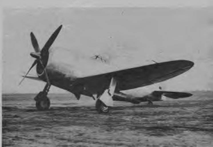
Army goes air-cooled. First 2,000 h. p. single-engine fighter is the XP-47B by Republic. Heavily armed and armored, it is said to have service ceiling of 8 miles.
