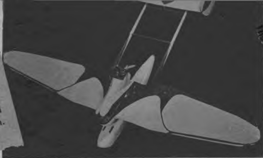
This tricky number features detachable outer wing panels, pusher engine, twin booms, kitchen sink—
