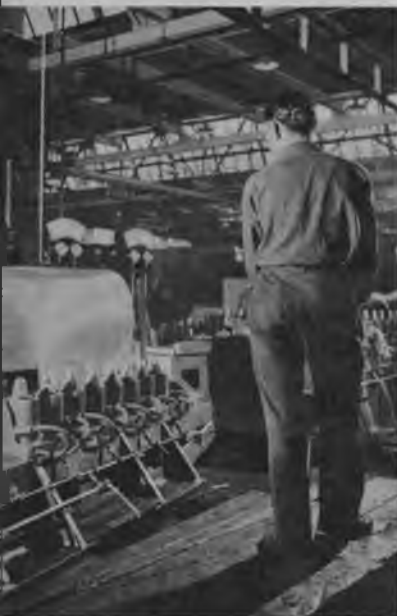
Jaws of metal-stretching press hold metal sheets; forms press up against them to form sections of covering.
