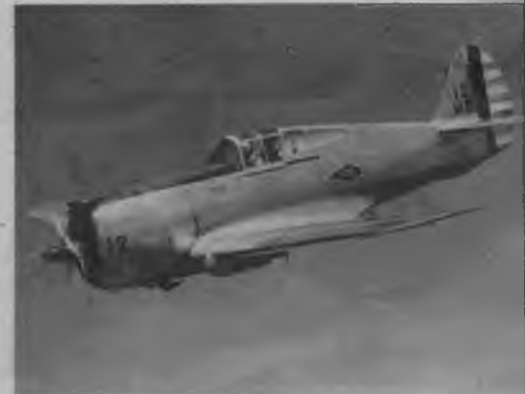
Still used here and abroad. This P-36A by Curtiss has speed of 323 m. p. h. and 1,000 mile cruising range.
