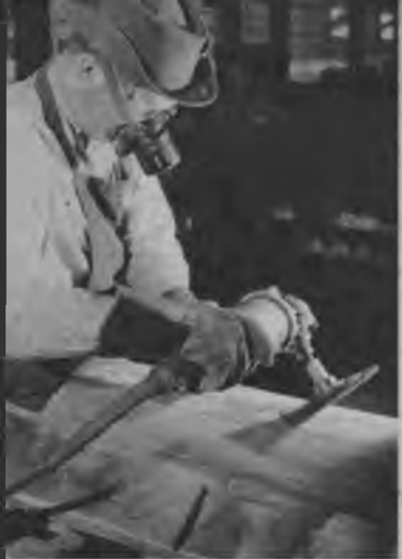
High shine. Zinc die destined for the drop hammer is ground to closer dimensions and polished for contour.
