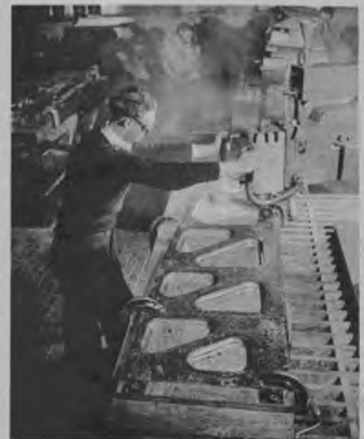
Intricate shapes are cut by power router. Eight to twelve sheets aluminum alloy are sandwiched between wooden patterns to serve as guide.
