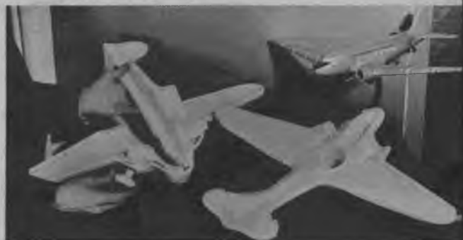
Plaster is poured around model to make casts. Casts are then duplicated in bronze for molds. White metal is cast in the bronze molds.
