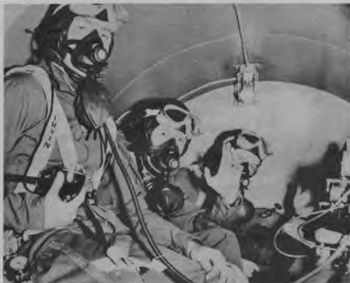
With nitrogen removed from systems pilots in Boeing altitude chamber are "flown" to 35,000 ft. Complete flying equipment is used in tests to simulate real flight.
