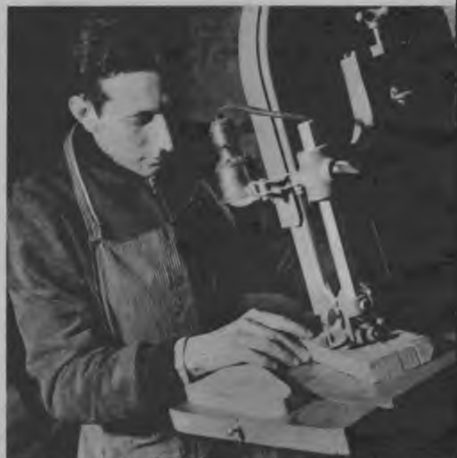
Sawing wood wing blanks for Stinson. After assembly carved blanks become pattern for plaster casts from which bronze molds are made.
