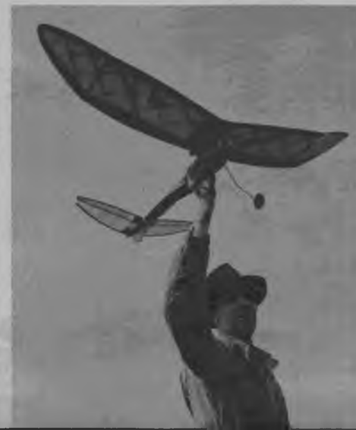
Geodetic wings distinguish Elmer Wassman's gas job. Spars are eliminated. On the whole, it looks a whole lot easier.
