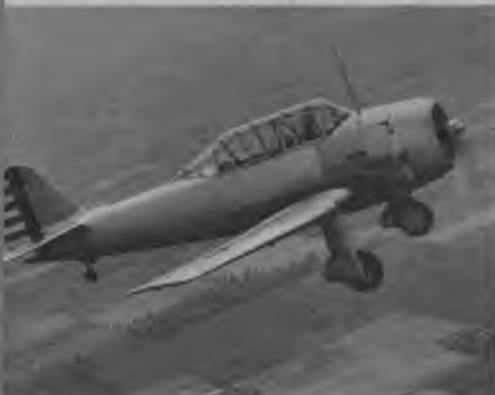
New basic trainer. Fleetwings XBT-12 has top speed of 195 m. p. h. Spot-welded steel fuselage gives strength.
