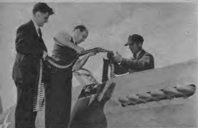
Loading up. Gun tests are a regular part of Wright Field routine. These experts are loading fifty-caliber guns in Curtiss P-40 for fire test.
