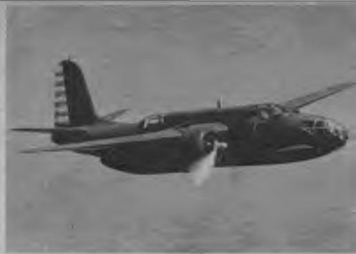
Twin-engine fighter. Douglas A-20A has speed of 325 m. p. h. Nose guns fire forward from streamlined coverings.
