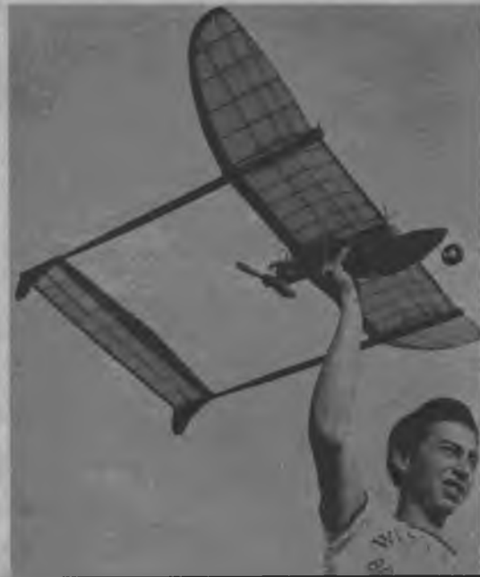
This Class A pusher is Robert Harrison's dream ship. Powered with a Megow 199, it flies well. One wheel and fin skids.
