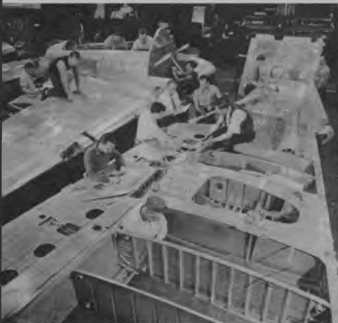
Pinions. Wings for the B-26 are assembled from many sub-assemblies and the smooth metal skin is fitted on. Installation of control wires, electric wires, "plumbing," and so forth, goes on from this point.
