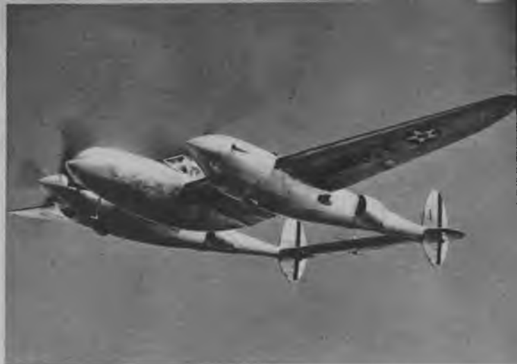
Our fastest production job, the Lockheed P-38, powered with liquid-cooled Allison engines has machine guns and cannon in center nose. Speed is over 400 m. p. h.
