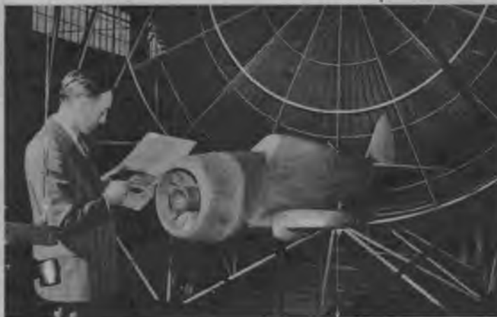
Final check. An engineer goes over a big scale model fuselage before test in the wind tunnel. Many of these models have movable control surfaces.
