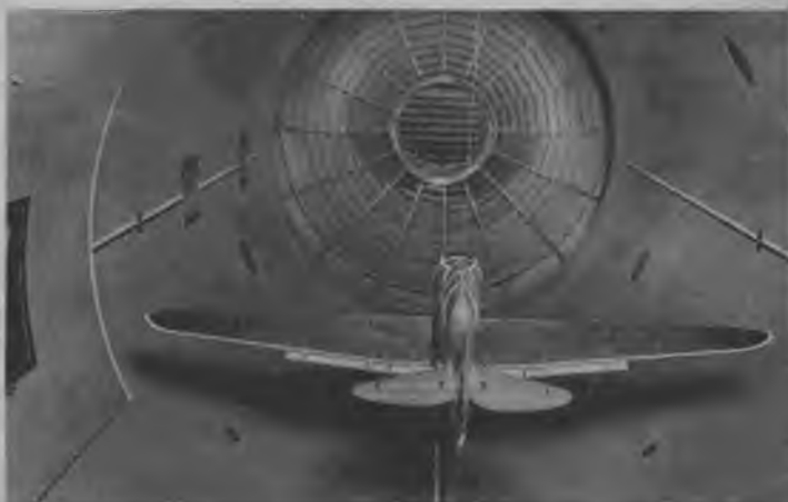
Sitting in a draft. The model with wing attached is suspended in tunnel ready for test. This particular model has scale flaps built in to test their effectiveness.
