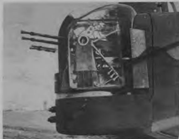
Behind the tail guns. Inside the four-gun turret in the tail of a Whitley bomber. Two guns on either side. Ammunition and triggers in center. Below—Side view of same turret showing the four guns. Sides of turret are of plexiglass for better gunnery visibility.
