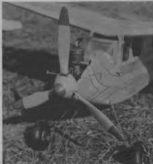
Centrifugal force holds folding propeller blades in position when the motor is running. Hinges must be strong for safety.
