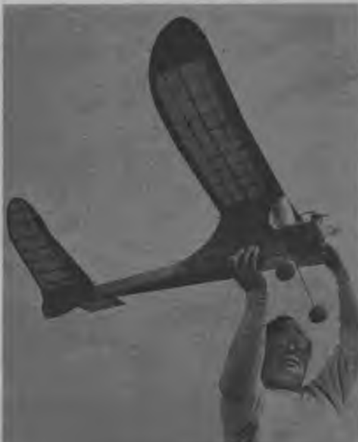
We like this one for its design. Crutch construction, sheet-balsa fuselage, "U" stabilizer, no rudder. Cliff Travis.
