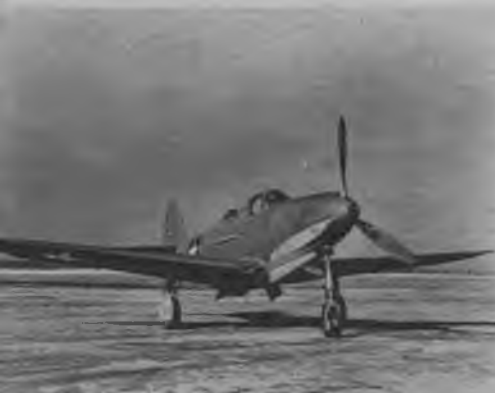
Giant killer. The Bell P-39 with Allison in rear of pilot has a shell gun in nose, as well as many machine guns.
