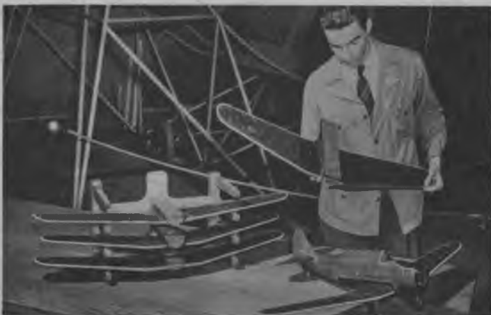
Now try this one. Various wing shapes are tried out on some fuselage model to determine efficiency of different wing designs. Tiny yarn tufts give data on air flow.
