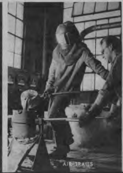
Man from Mars? A melter pours hot metal to be transferred to small sand molds for drop-hammer dies.
