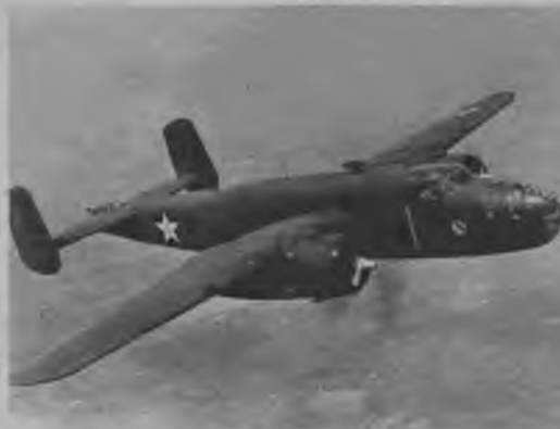
Twin-engine bomber. The North American B-25 has a speed of well over 300 m. p. h. Note the tail turret gun.
