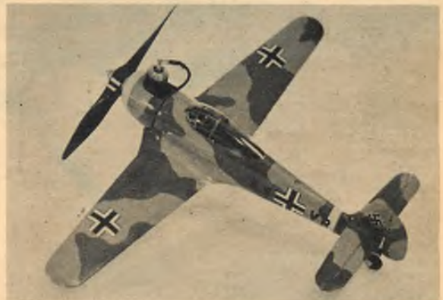
● Arden ignition .099 powered FW-190 built by Ed Callahan, Chandler, Okla. Carved balsa; numerous coats of dope.
