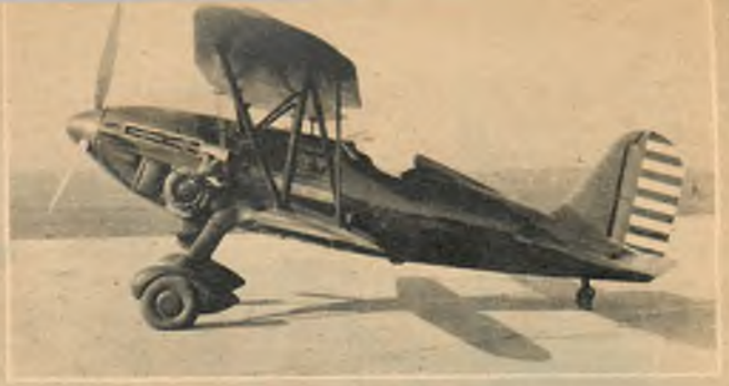
● XP-23 was the last Army biplane Hawk. Converted from a P-6E, it had a metal monocoque fuselage, cantilever tail surfaces, was equipped with turbo-supercharger. P-6E contract completed Christmas, 1933. Many were still in service in '41.
