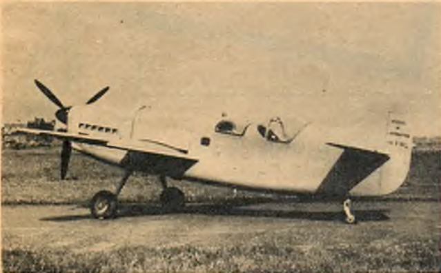
● Arsenal O-101 French two-place research plane. Observer sits ahead of pilot. Engine 495 hp Renault, speed 280 mph.
