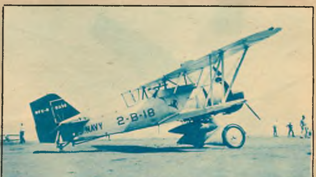
● Navy's last series of Hawk, the BF2C-1, 28 of which were ordered. Model was further developed and built for export under designation of Hawk III and IV. Total number of Hawk biplanes built for Navy: 132. Last Hawk IV sold to Argentina.
