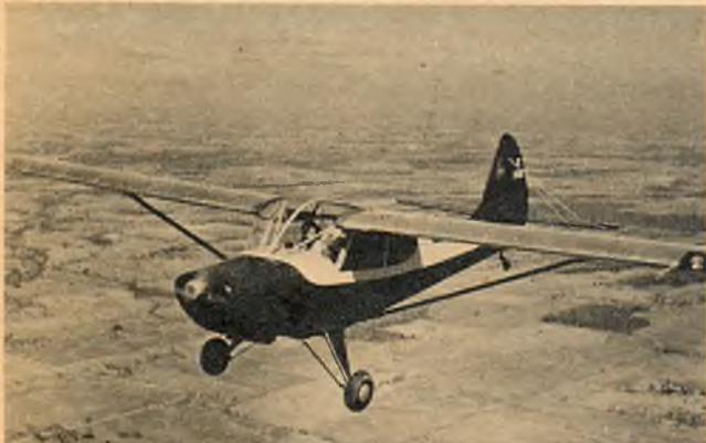
● The Sedan, Aeronca's entry in the four-place personal plane field. Span 37' 6", engine 145 hp Continental, speed 120 mph.
