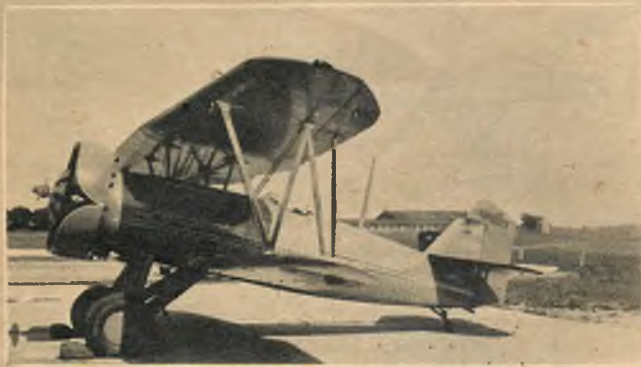
● Hawk 1A designation was assigned to commercial and export model developed from basic P-6 powered by a Wright Cyclone and known as YP-20. Numerous Hawk 1A's bought by foreign governments. Most famous of all was Al Williams' Gulfhawk.
