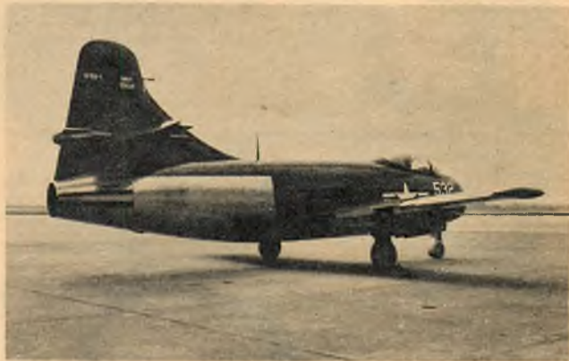
● Chance Vought XF6U-1 Navy fighter now has an after-burner to increase thrust. Rear of fuselage modified for device.
