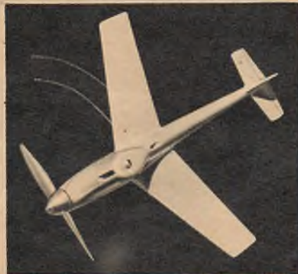
● Lt. (USN) Ed Baker's Class D Hassad ship with supersonic airfoil; span, 19½".
