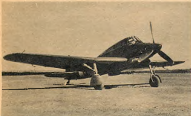
● Italian SIAI Marchetti SM 93 dive bomber developed at close of war. Pilot lies prone. Top speed 337 mph, wing span 27'.
