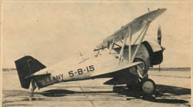
● BFC-2 was the designation given to the F11C-2, 26 of which were ordered. One model of F11C-2 was converted to XF11C-3 by modifying the nose and fitting plane with retractable landing gear. This modification raised plane's top speed to 216 mph.
