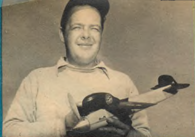
● Charles W. Mathews, Alameda, set record of 150.57 with his Hornet-powered ship. Length, 19"; span, 18"; 26¾ oz.
