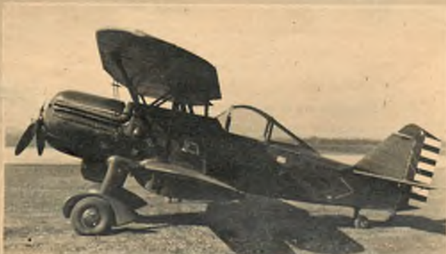
● XP-6F, equipped with turbo-supercharger and cockpit canopy. The Conqueror engine developed 675 hp. The plane was 6 mph slower than the P-6E at sea level, but at 15,000 ft. it topped 220 mph, the fastest of Army or Navy Hawks at that time.
