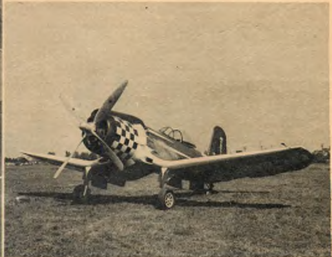
● Cleland's winning plane, the F2G Corsair, specially re-built for the race. One of modifications was FG-1 tail.
