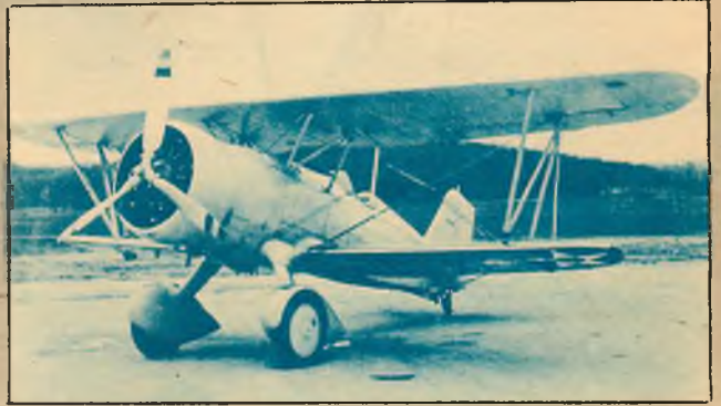
● Navy XF11C-1, powered by Wright 1510 engine, 600 hp. Designation later changed to XBFC-1 under Navy's multiple purpose classification and plane was classed as bomber-fighter able to carry 500 lbs. of bombs under either wings or fuselage.
