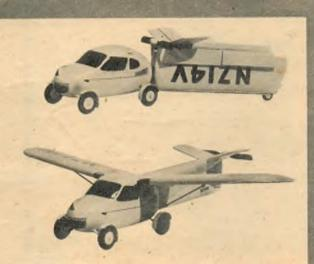
Taylor's Aerocar: Tail and wings form trailer. Trailer wheels built into leading edge of wing at root. Car unit has already been built and tested, proved very satisfactory.
