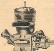
DOOLING "61" For highest performance in race cars, planes, boats. Still the finest, most powerful engine for its displacement ever built. Roller bearing connecting rod-.607 cu. in. displacement-rotary valve, plate type-weight, 14 oz.
