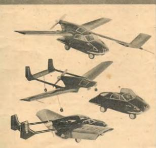
• William Chana, Consolidated-Vultee engineer, designed this flying auto which can be converted into pusher plane, canard or helicopter, using same car. 'Copter not shown.
