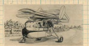
Projected roadable airplane design by Henry Clark. The entire aircraft component is carried by the vehicle, securely latched to the roof.
