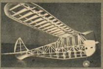
Philadelphia's Edward V. Hess, Jr., designed this Class D free-Right for Ohlsson 60 Ignition flying. Weighs 68 ox.; span, 90; area, 990.
