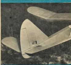
Simple installation of escapement is evident from this shot of the rudder. Note stab dihedral
