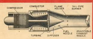
Afterburner: raises jet temperature, lifts turbojet thrust.
