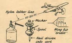
Used plastic margarine bags, washed with soap and hot water, make ideal containers for dust-moisture-proof storage of engines, says Herman Hadsall, Des Moines, la.  Small models, midget gas or CO<sup>2</sup> can be flown tethered indoors. One way is method of Robert McKone, Hartford, Conn. Use water-filled jug. Short lines work well.
