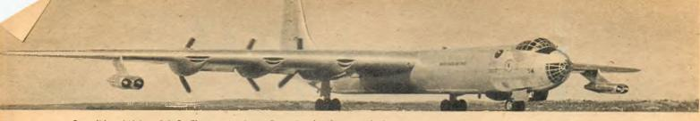
• Consolidated-Vultee B-36D: The mammoth Air Force bomber has been equipped, in addition to its six 3,000-hp reciprocating engines,
