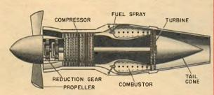
• Turboprop: capable of developing in excess of 10,000 hp.
