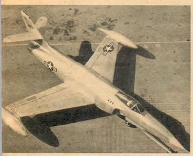
• Lockheed F-90: Air Force's latest penetration fighter, powered by two Westinghouse J-34 jet engines of 3,000-lbs. thrust each. Wing span is approximately 40 ft., fuselage length 55 ft. Wings have 35° sweepback, and are extremely fhin. Speed over 650 mph.
