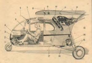
• Cutaway view of Clark's roadable: 1—clutch, 2—accelerator, 3—foot brake, 4 headlights, 5—control wheel (ground and air), 6—pitot tube, 7—hand throttle, 8—wing support peg, 9—aileron push rod, 10—air duct, 11—wing lock fitting, 12—zippered gap flap, 13—prop shaft uncoupling and drive unit, 14—lower drive unit, 15—universal joint, 16—clutch housing, 17—strut bolt.
