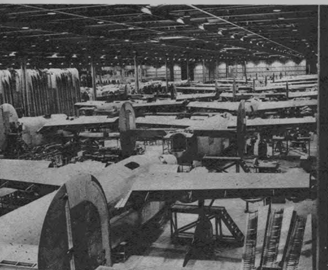
By day and by night B-24's come off the line. This night shot shows the big long-range four-engine bombers being assembled by the night shift.
