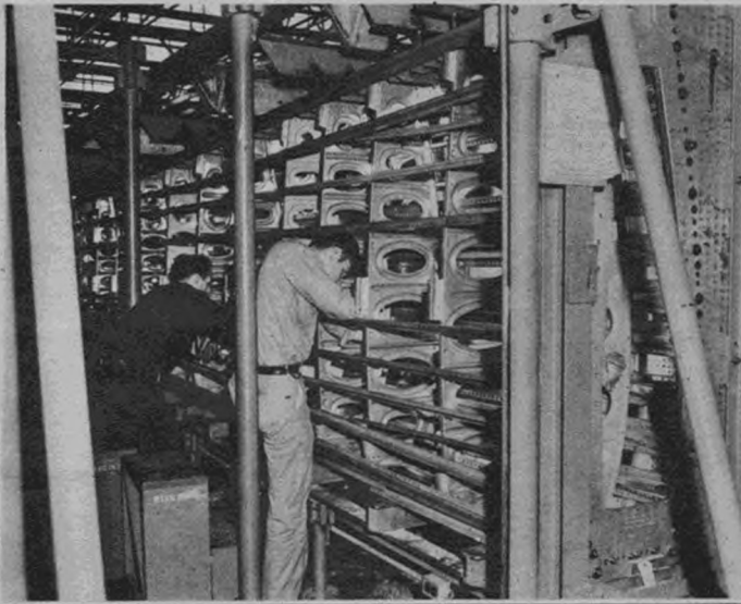
Frozen assets. Portable ice chest keeps rivets chilled until ready for use. They are kept from 0 to 25 degrees below zero until used to prevent splitting when driven.
