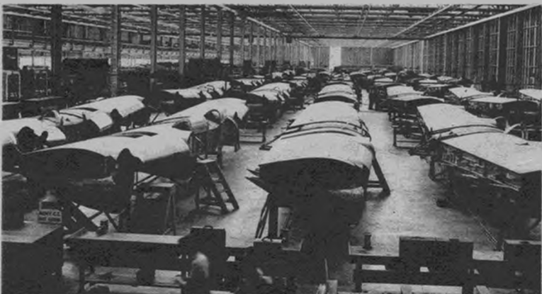
Coming right behind. Back in the plant more B-24 wing center sections are going together. Note engine nacelles under wing panels for four 1,250 h. p. P. & W. engines.
