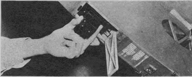
Hinged trapdoor opens automatically when Auto-Knips timer cuts motor. Small bakelite camera shoots 35-mm. film. Its weight is negligible.
