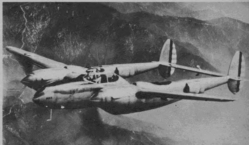
Our Lockheed P-38 supercharged twin-engine single-place fighter, with a speed well over 400 m.p.h., is one of the world's best ships in this category.
