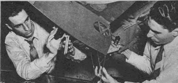
Oliver Pfeil, left, and his brother William built this Comet Clipper camera model. The one-wheel landing gear saves weight and cuts drag.
