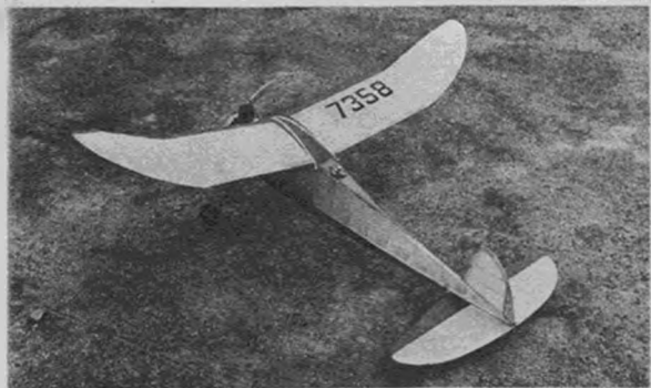
You can't beat the Request for climb. Won't loop, even when it is so adjusted. Teardrop fuselage section cuts drag in climb.
