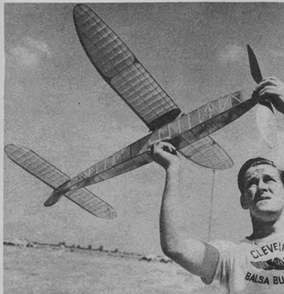
Korda found gas-type pylon caused model to drift out of sight too fast in windy weather. Note the multispan wing and tail construction.
