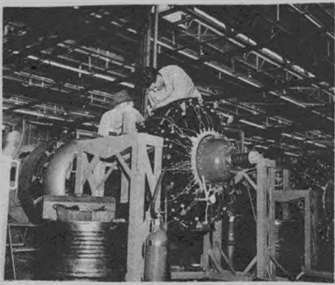
Out of the crate, the engine is checked and given inspection before being installed in its mounting.
