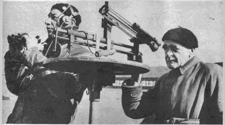
With the aid of this complicated spotting scope the range, height and speed of the invaders are computed. Instrument rotates to follow flight of enemy planes.
