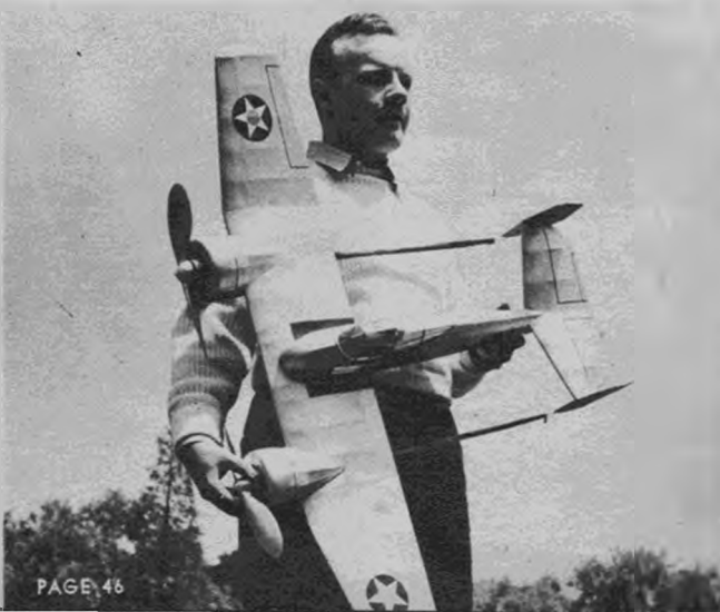
Two twelve-inch props turn in opposite directions to counteract the torque.
