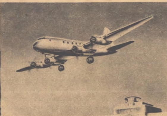
Handley-Page Hermes V with four Bristol Theseus engines
