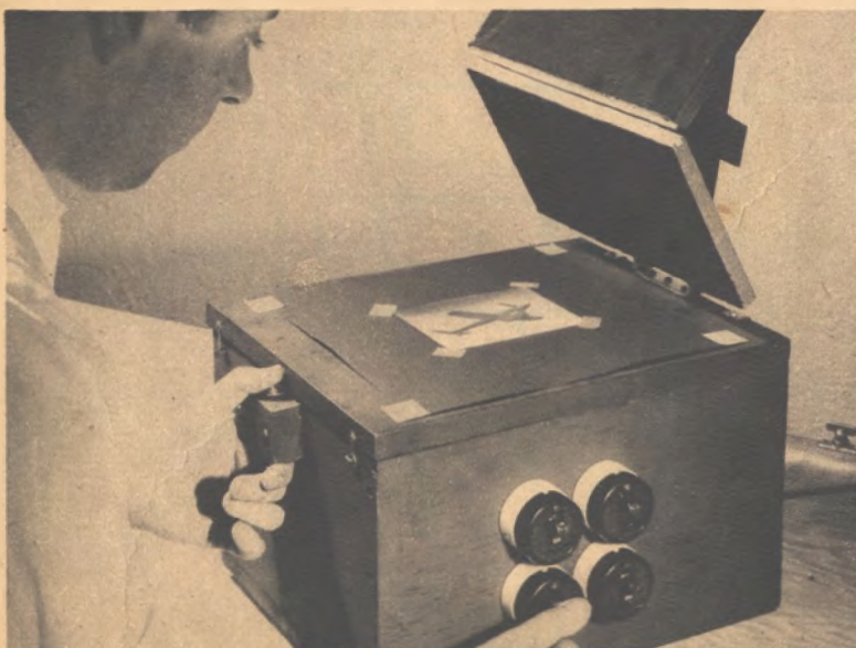
● Individual switches permit light control to portions of negative.
