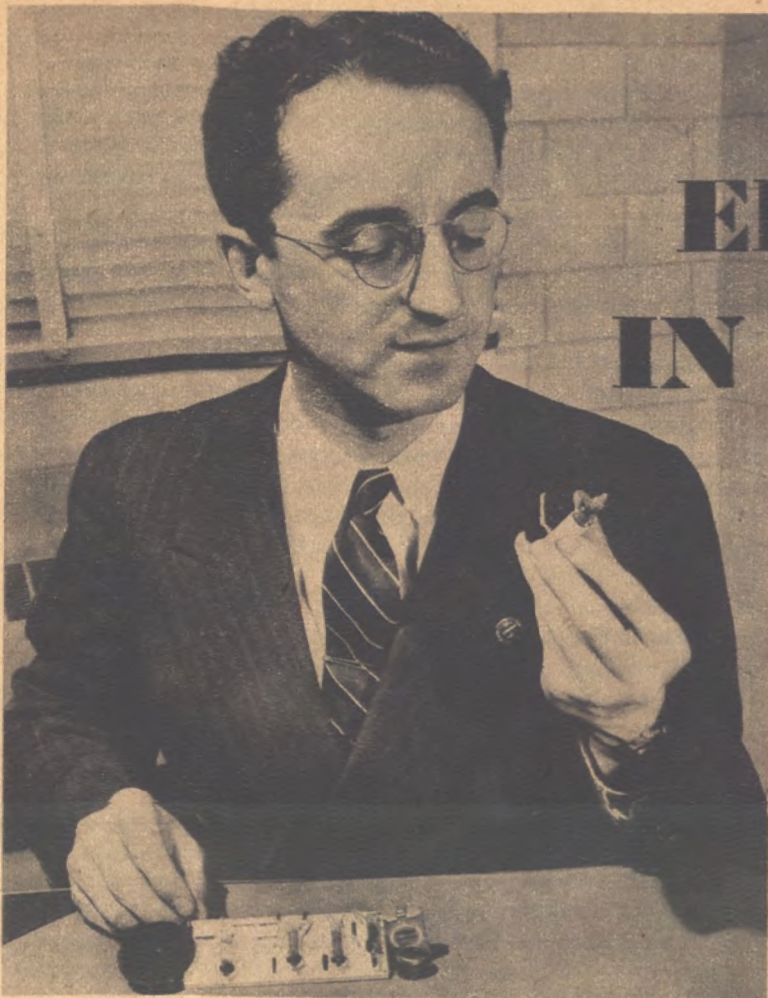
● Dr. Clelio Brunetti of the National Bureau of Standards examines a transmitter complete with batteries and microphone. A receiver is on the desk.
