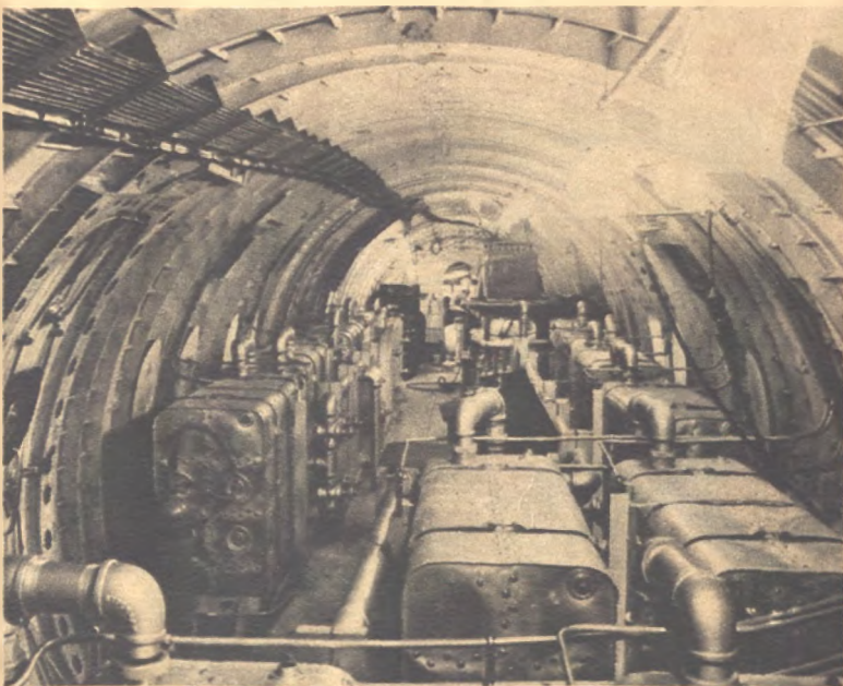
● Water ballast tanks permitting transfer of loads to different parts of the airplane in center of gravity tests, were first developed by Lockheed.
