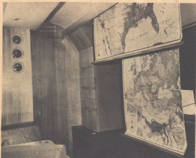
● Above. President's-eye view of executive stateroom. Flight instruments at left, built-in wardrobe, and maps pulled down from recess in the ceiling.
