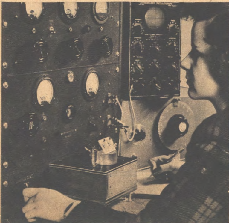
● A sub-miniature amplifier gets put through its paces at the Bureau. Performance of the tiny unit is practically equal to conventional types.
