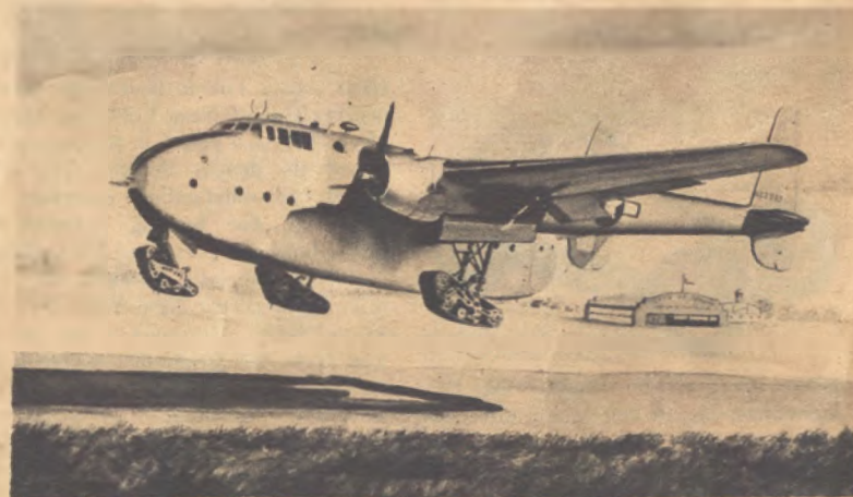
● Fairchild Packet equipped with tractor-type landing gear which will enable the craft to operate from sand, mud, and unimproved landing strips.
