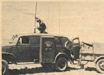
● Tech. Sgt. G. Howland installing antenna on SCR 299 radio unit of Essex Squadron.
