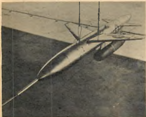
● Martin Gorgon IV guided missile fitted with Marquardt 20" ramjet.
