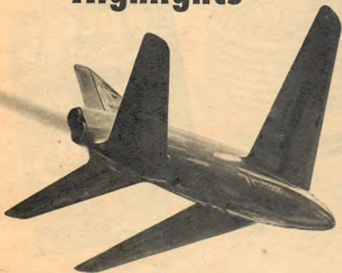
● Exhibited at recent air show in Paris was this 11/28th scale model of French SE 2410 jet attack plane, now under construction. Powered by two RR Nene engines mounted one above other.
