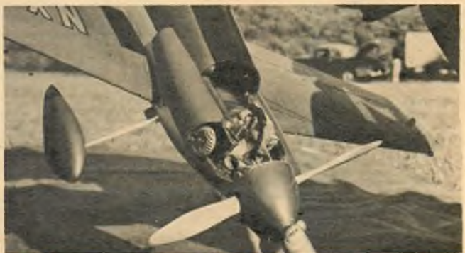
● Power department of model Long Midget. Ohlsson 29 was used on author's model, but motors up to .40 cu. in. displ. are possible.
