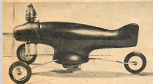
• Like Texas, this ship is big! Galen A. Stephens of Austin Aerocrats with original Orwick 64 powered 8-ft. job. Chord, 12 in.; area, 1,072 sq. in.; wt., 65 oz.
