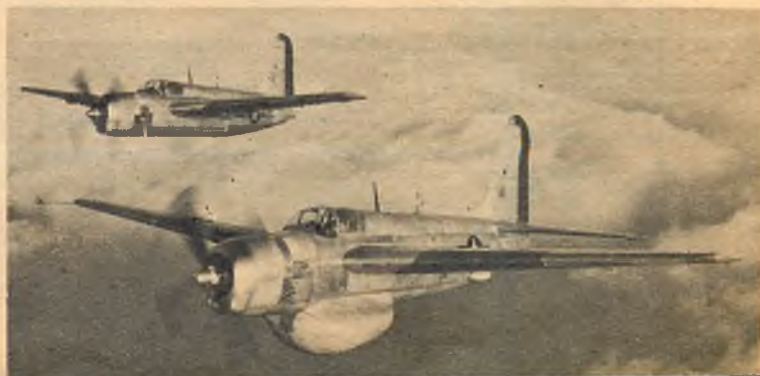
● Navy's newest anti-submarine aircraft, the Grumman XT83F-1S (top) and XT83F-2S. Production planes will be designated AF-1S and AF-2S and called the Guardian. Bulge under fuselage is large search radome. Both have Pratt & Whitney R-2800 engines.
