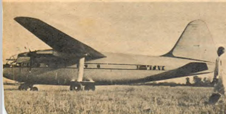
● French light-freighter the Fouga CM-100, a development of the Castel-Mauboussin CM-10 glider. Can carry a maximum of 21 passengers or an equivalent weight in freight. Is powered by two 580-hp Renault engines. Span 84.3 ft. Speed 187 mph.
