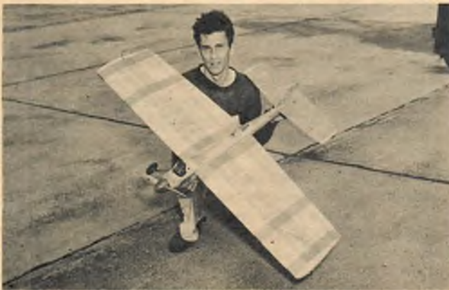
● Plymouth International stunt champ Lew Andrews of Boston, Mass., flew his new design. Wing has 660 sq. in. area, weighs 2 lb., 7 oz.
