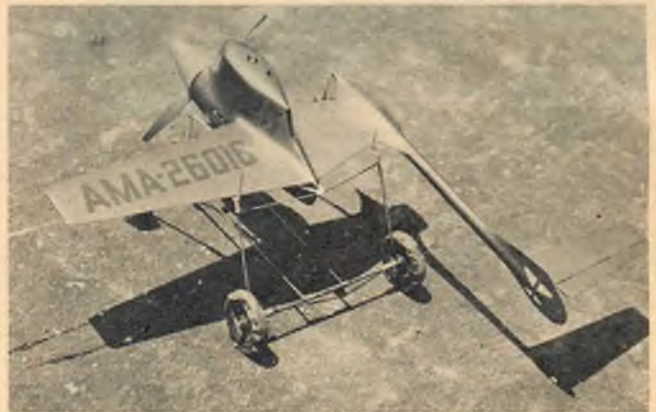
● McCoy 29 powered asymmetrical speed job entered by J. Warren Kohler. Speed events were timed by electronic-operated pylons.
