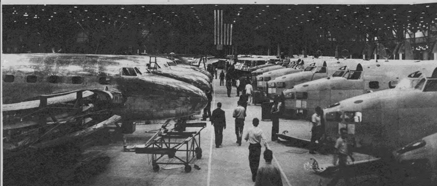
Peace and war. Two production lines in the 600-foot final assembly hangar show on the left the Lodestar transports and on the right the Hudson bombers. These
