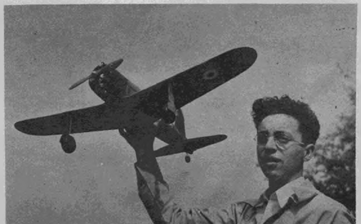
This baby Vanguard is built one-inch-to-the-foot. A Super Atom engine is used, but any Class A or B motor will do. Size of engine affects speed accordingly.
