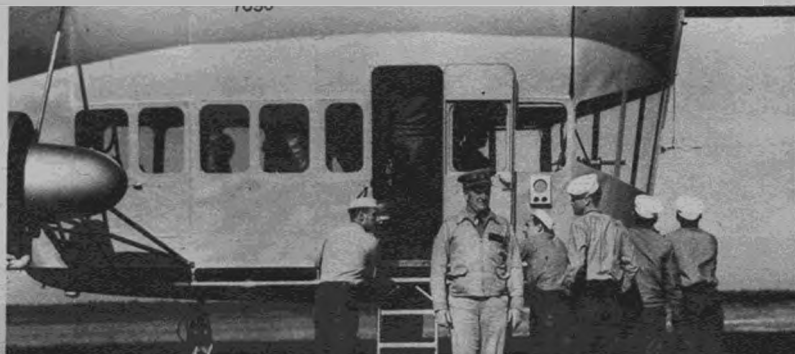
The author and the good ship K-2, a nonrigid of 400,000-cubic-foot helium capacity. The blimp's duration, ability to hover, and 8-man crew make it effective for coast patrol.
