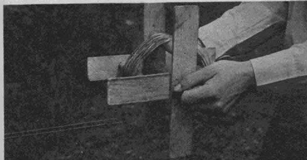
A homemade wooden hand reel is needed for winding the control wires when not in use. Unless such a reel is used music-wire lines may snarl.
