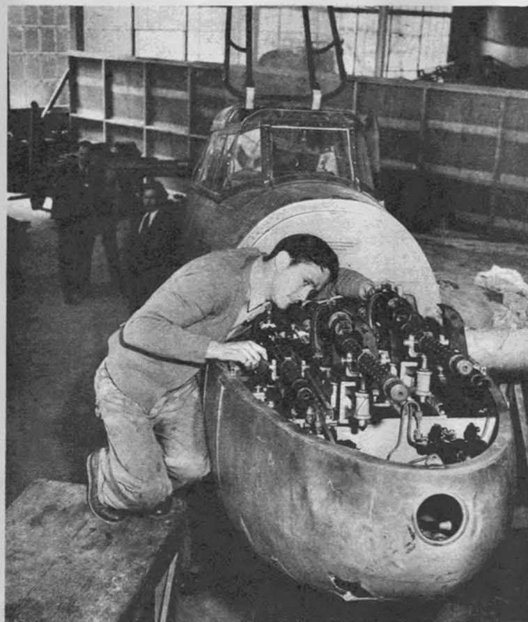
Vultee worker examines fallen Messerschmitt 110 shipped here by British. Four guns shown are .30 cal. Hole in nose is for camera. Two 20-mm. cannons fit under nose.
