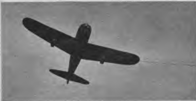
Roaring overhead at 50 m. p. h., our model Vanguard reveals control wires that run from operator's hand grip to the ship's control mechanism.
