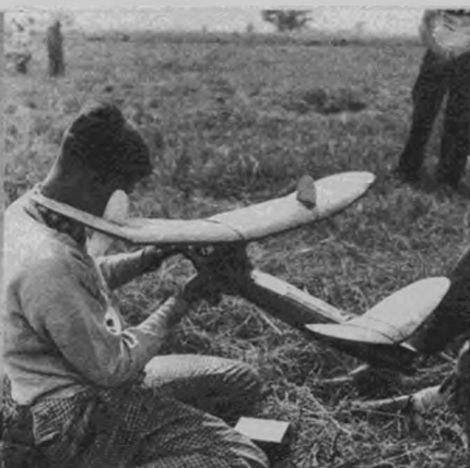
Pusher canard, by Jack Leredahl, was soundly designed, well worked out. Note wing fins.
