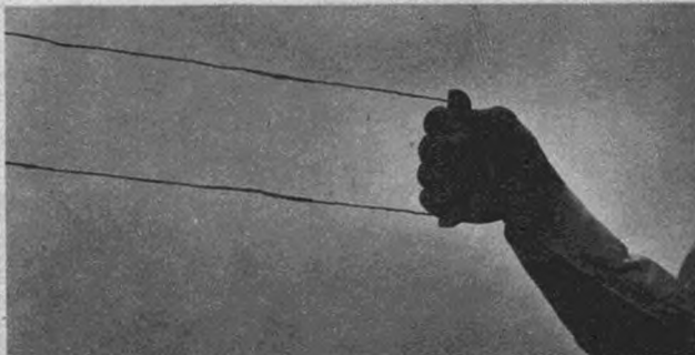
The control method is adapted from the patented "U-Control." Tipping the top of stick forward causes ship to dive; pulled back, model climbs.
