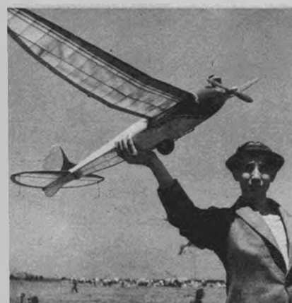
"Clean lining" is the word for it. Planked fore fuselage, longerons aft. Schoenfeld.
