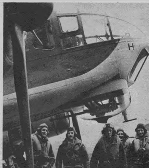
Aimed by remote control, machine gun in tricky turret on Beaufort torpedo-bomber gives increased protection.
