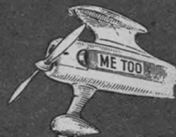
Modified Sailplane, by Ellis; planked, and faired wheel.
