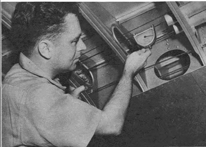
After assembly every part is carefully checked for perfection and compliance with the specifications. Here the tension of a control cable is being very carefully checked.
