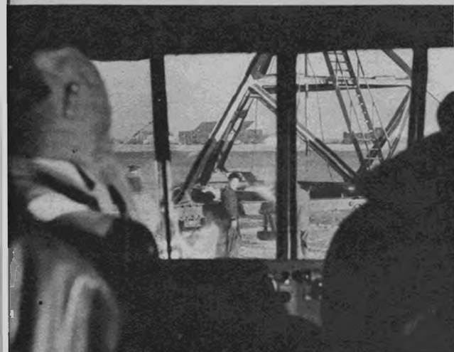
The crew awaits the take-off signal. Engines are warmed up as the blimp strains at the portable mooring mast.
