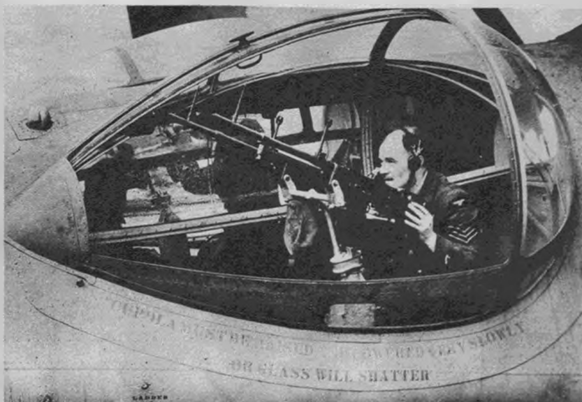
Ready for all comers. Rear gunners on Consolidated PBY-5s (Catalina in England) man two sets of these swivel-mounted machine guns. Huge blisters designed on basis of war findings.
