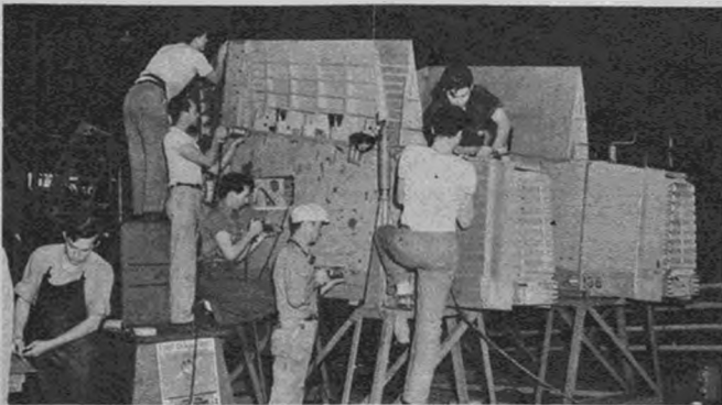
On castered dollies these wing-center sections progress down their individual assembly line. Here a riveting crew fills in its part of the job.
