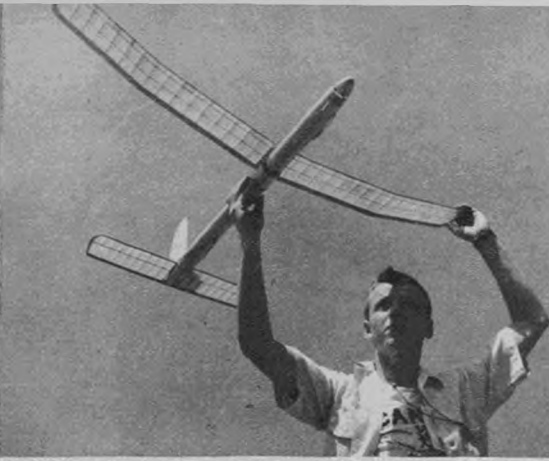
One of the nicest stick jobs we've seen. Tubular stick from 1/32 -inch sheet balsa, high-aspect wing. By Caldwell Johnson.
