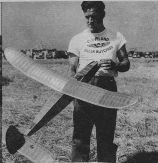
Dick Korda was the man to beat. Took first in Class C Open in rubber. 300 sq. in. job had timer dethermalizer.
