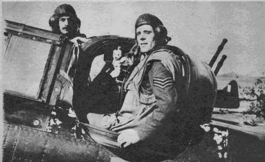
Famous multigun power-operated turret on Defiant night fighter can train its guns up or to the side at right angles against strongest slipstream. This crew has thirteen victories.
