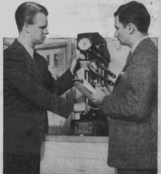
Checking the hardness of metal after welding, using a Rockwell Hardness Tester, an example of the fine equipment provided for student use.
