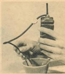
Pressure regulator valve tested with siphon tube for correct opening-closing pressure.
