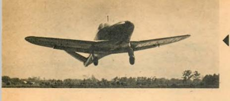
With flaps in maximum lift position, Jupiter hops off at 45 mph after not more than 300-ft. run. As soon as gear is tucked in place she accelerates fast.
