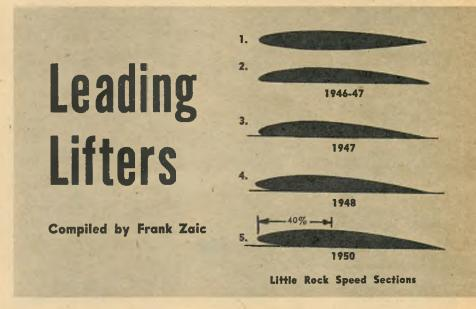
goes from 1946 streamline to 1950 streamline in front of 40% and Clark-Y-ish towards T.E. He mentioned that streamlined or similar sections tended to do a "high speed mush" at times—while present section indicated sharp improvement in lift, lower drag and stability at high speed. He also believes that it makes trimming easier and provides good lift at landing speed. Used in combination with streamlined stabilizer with 1½ deg. difference, and rectangular planform.
