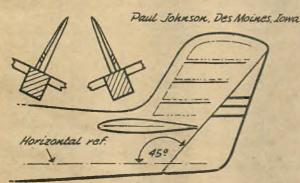
R.C. model rudder with swept hinge line imparts upward movement for safe turns
