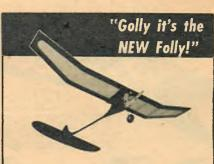
"FOLLY" 1/2A FREE FLIGHT for all Engines .035 to .074. Wing span 32", 5" chord. Wing area 146 sq. in. Prefabricated and designed for contest performance, yet simple and easy enough for the beginner to build & fly. R.O.G's
