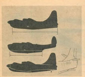
Three silhouettes show difference in hull length between Martin PBM and new PBM-1 (second figure). Hull flap shown in bottom corner greatly increases plane's taxiing maneuverability.
