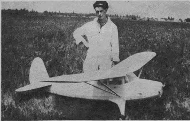
This lifelike Fairchild monoplane was built by Alfred Rusher of Olympia, Washington. Wing span is 8 feet 8 inches. Motor a ¼ h. p. James.
