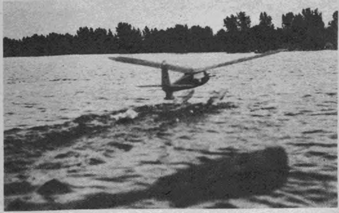
Over the waves. Joe Dellaire's 9-foot webfooted gas job takes off at a Detroit hydro contest. Note how model is planing on pontoon steps.
