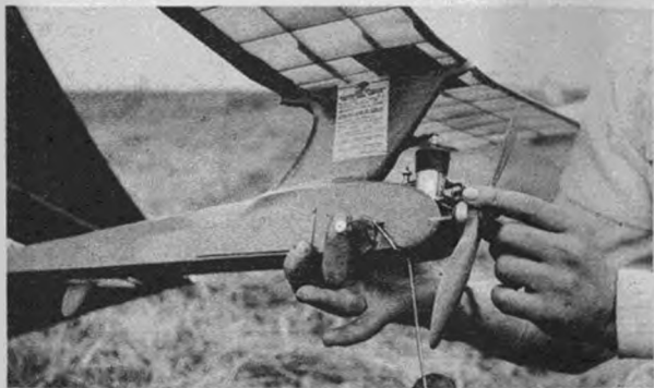
This Interceptor typifies the modern layout for high climb, efficient glide. Even wheel retracts.
