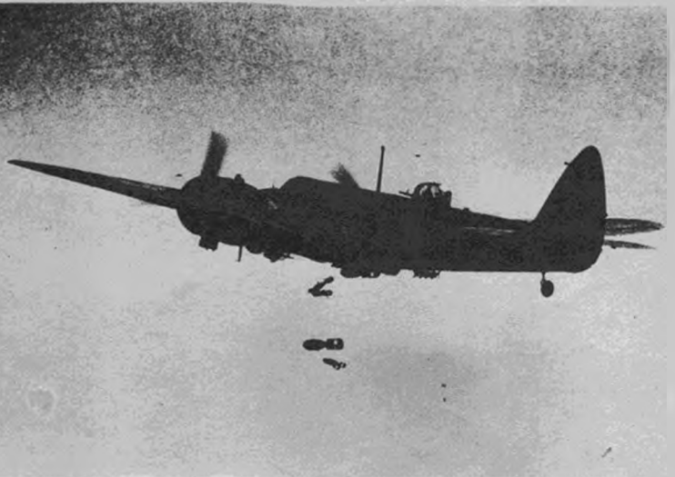
This stick of bombs being released over Vichy by R. A. F. plane shows method of dropping. Smaller bombs are dropped from wing racks; big ones from within.
