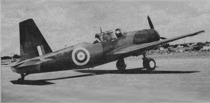
Newest dive bomber. This Brewster Bermuda carries 1,000-lb. bomb within fuselage. Has twice range of German types, powered turret.
