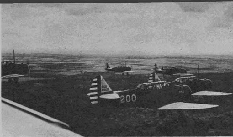
Over vast Texas plains wheel training formations of BT-9s. Partly open wing slot in left foreground preserves smooth flow of air over tip at steep flight angles.
