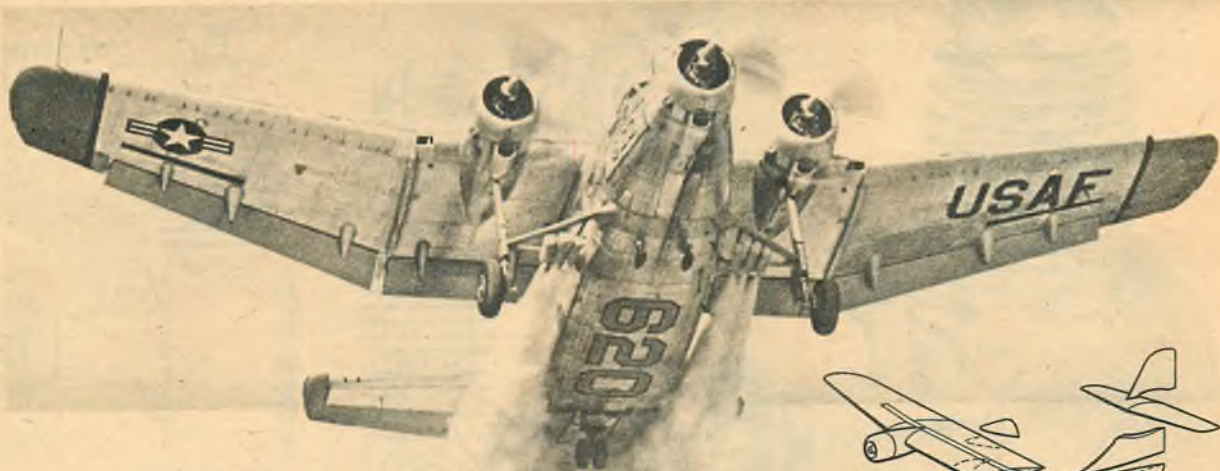
Air Force's new "light" assault transport uses six Jato rocket units to help lift its 40,000 pounds over obstacles
