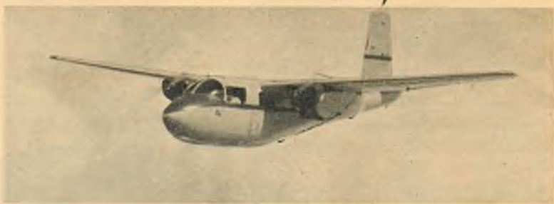
Aero-Commander by Aero-Design & Engineering Corp., Culver City, Calif. A new executive transport. Span 43'10"; engines two Lycomings, 190 hp each.
