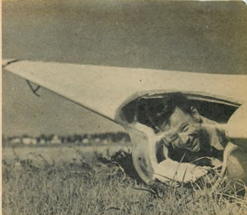
fabric reinforced plywood. Pilot has to extend arms in wings to control craft. Tail cone fits over occupant's legs. Span 25'4", length 7'4". Was not flown. All control surfaces are at the wing tips.
