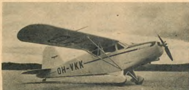
Kahru 48. Finnish four-place personal plane designed to be used on wheels, skis or floats. Powered by a 190 hp Lycoming engine. Span 37'10", length 25'9". Speed 140 mph. Range over 400 miles.
