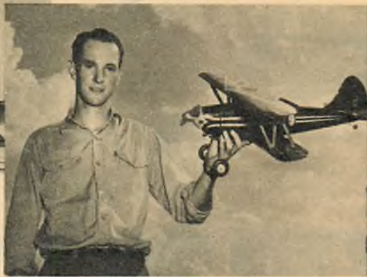
Howard Thoms, Warren, Ohio, won new Testar best-finish perpetual trophy with semi-scale biplane. Plane has K&B 32 Glo-Torp, 325 sq. in. of wing area, weighs 21 oz.
