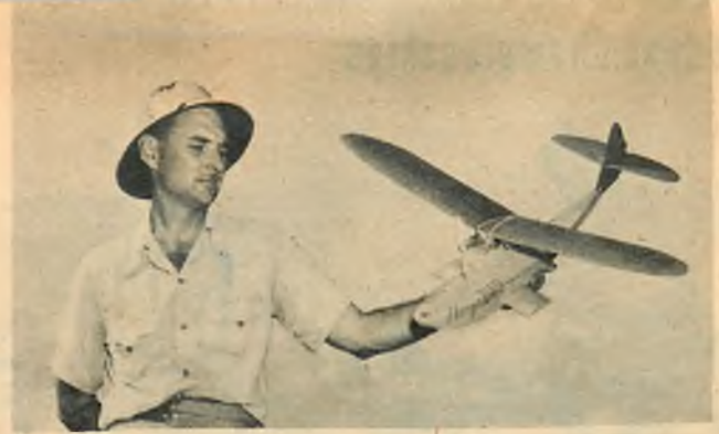
Bob Holland, '48 Nat. Champ, holding Art Snyder's Wasp-powered seaplane. Ship weighs 7 oz., has 150 sq. in. of wing area, reports Bob.
