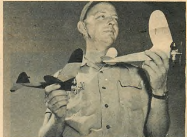
K&B's Lud Kading with "Gnats." Without engine one on left weighs 2 oz., has done 17 mins. with .02 infant. Boasts 21 sq. in. area.
