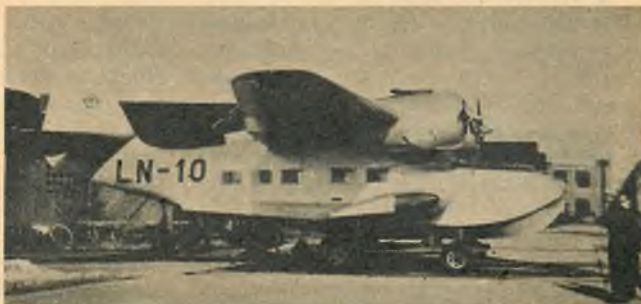
Finnmark 5A. An all-metal Norwegian flying boat specially designed for Arctic climatic conditions. Carries 14 people. Span 55'9". Engines P&W Wasps of 600 hp each. Maximum speed, 190 mph.
