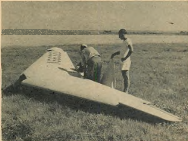
Flying Wing Sailplane designed by Vanderbilt U.'s Franklin Farra, shown in cockpit on the right. First exhibited during National Soaring Meet in Texas. Construction is entirely of wood, covered with
