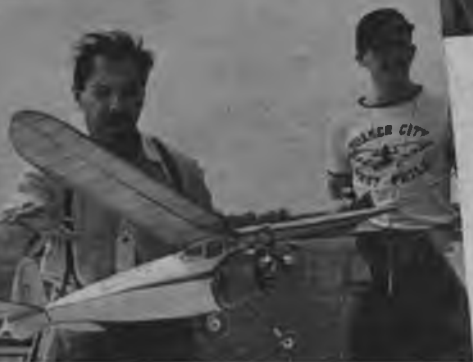
Above—Garami and the Molecule. Left—Start of the record flight at Hadley Field, where the Molecule outflow larger ships. The monocoque fuselage and wing installation are points to note. Nose detaches.
