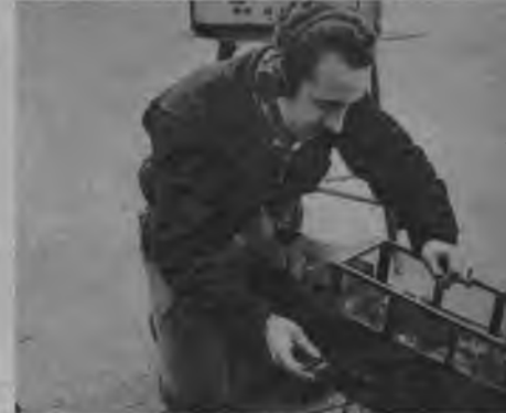
Middle—Close-up of receiver and selector units. The receiving set weighs 15 ounces. Right—Tuning the receiver to the 5-meter ground transmitter. A bakelite screw driver is used to adjust the condensers.
