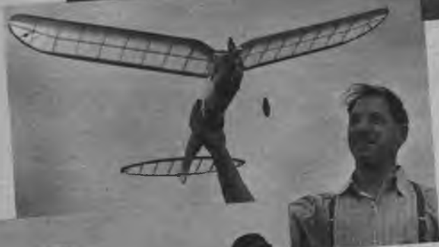
Above—Garami and the Molecule. Left—Start of the record flight at Hadley Field, where the Molecule outflow larger ships. The monocoque fuselage and wing installation are points to note. Nose detaches.
