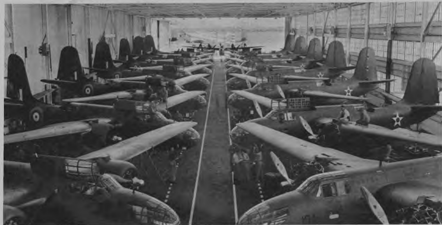
One-way street. Here American and British production lines carry DB-7s down Douglas City street and out the door for flight testing from field beyond.
