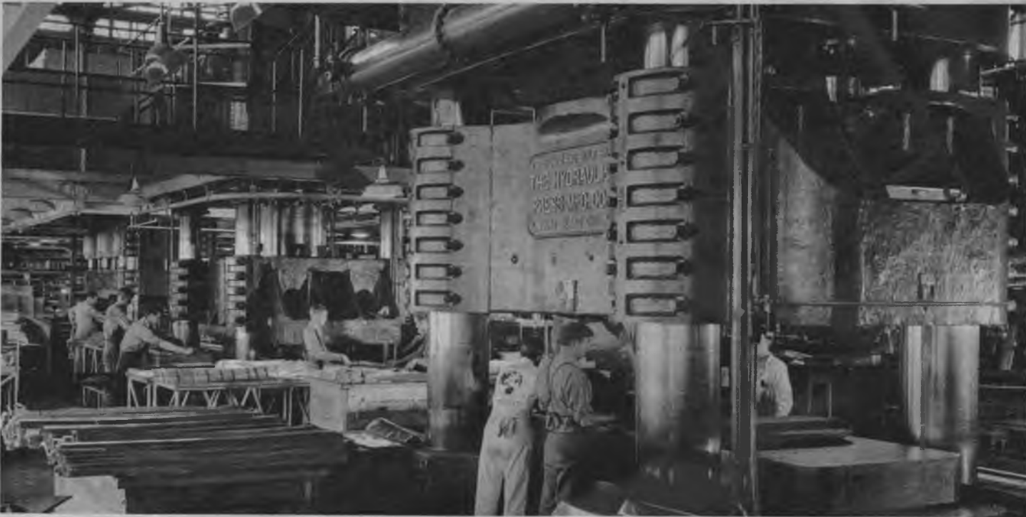
On one particular street of Douglas City are three of the four giant hydraulic presses developed by this company. They press over 44,000 parts a day.
