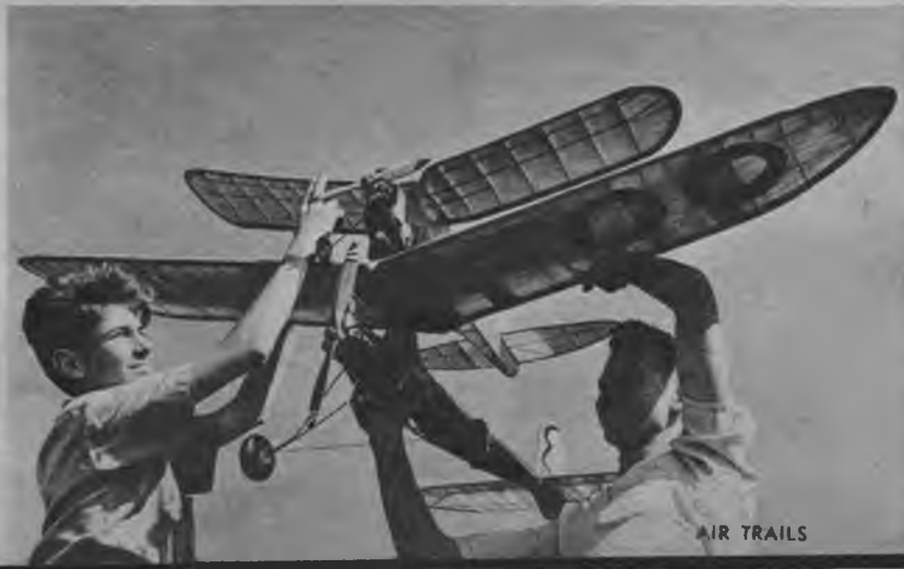
Not to be outdone by Vincent's pickaback, Bill Oberbeck and Tom Green teamed up two gas jobs. Timer on small ship is set for longer motor run than bottom model.
