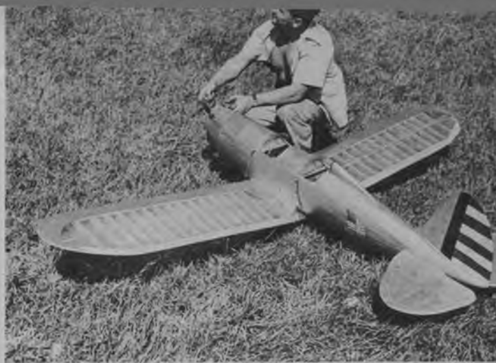
Not a real plane that dropped in at the contest, but a huge 8 1/2-foot Ryan scale model by Kerson Bologh. Motor is an Ohlsson 60. One trainer the army missed.
