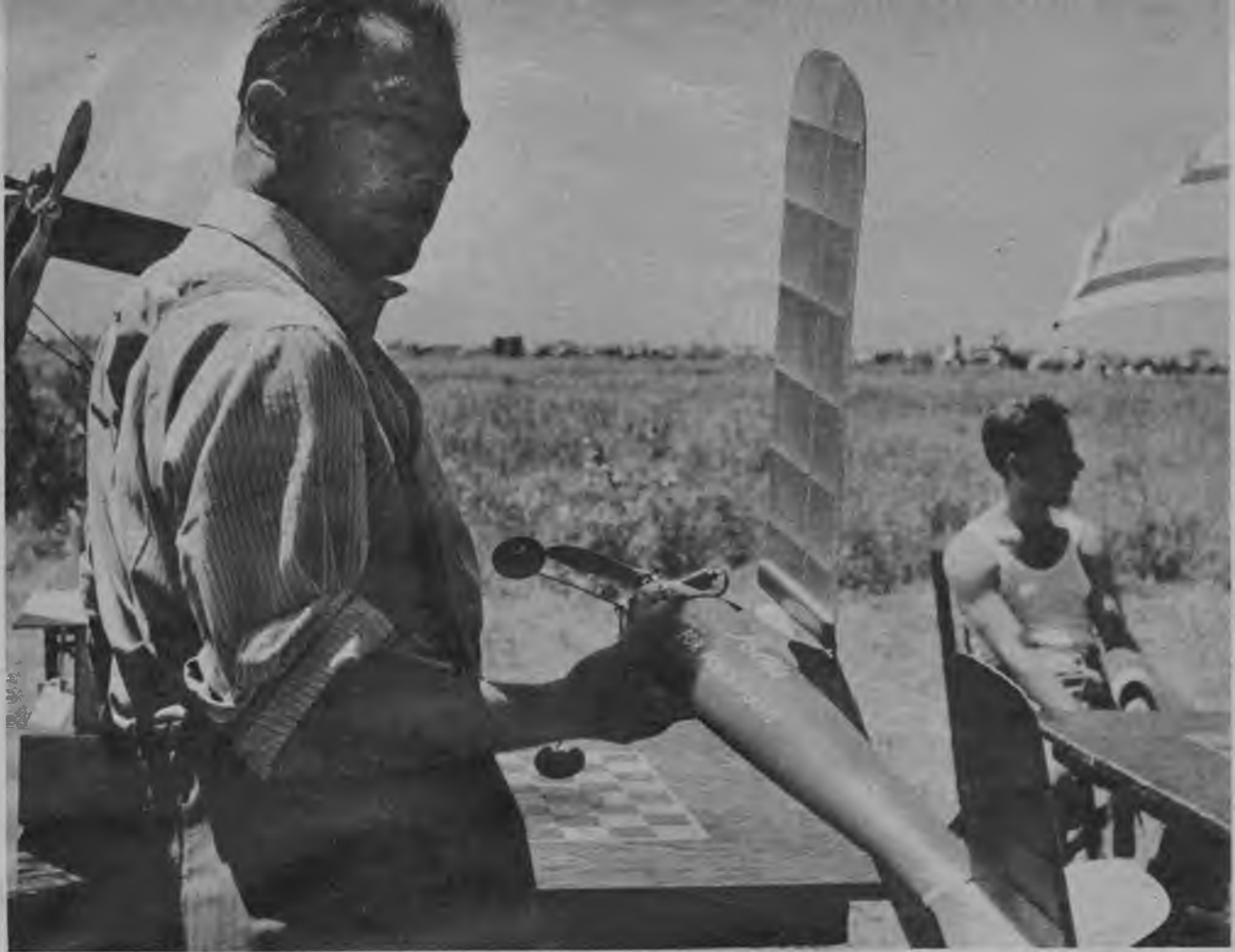
Louis at the Nationals with one of his all-balsa-fuselage gas models. The sheet wood is bent to shape by the simple trick of doping it on one side.
