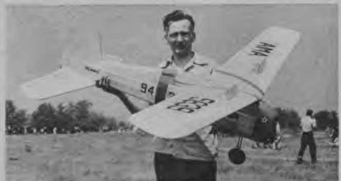
Out-of-sight squawkers look over these spoilers on wing of W. A. Manes Apache. Worked by timer, they kill lift, boost drag, to bring down ship.
