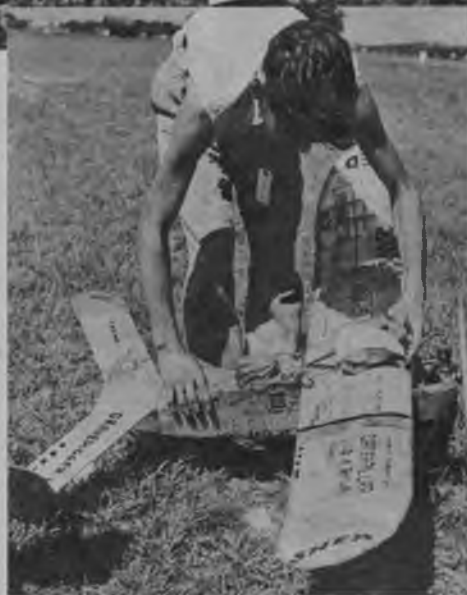
Paper holds down pilot chute. Free, paper blows back, releasing small chute, which pulls out large one.
