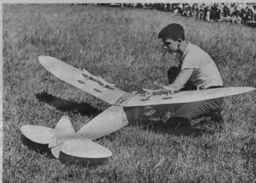
We'd hate to have to watch all these models at the same time. Timer pulls pin to release two gliders at once. Mother ship carries total of six. Jim Wood deserves a hand.
