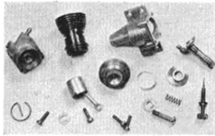
The Cobra engine broken down into its component parts. Note the cylinder head with its integral glow filament.
