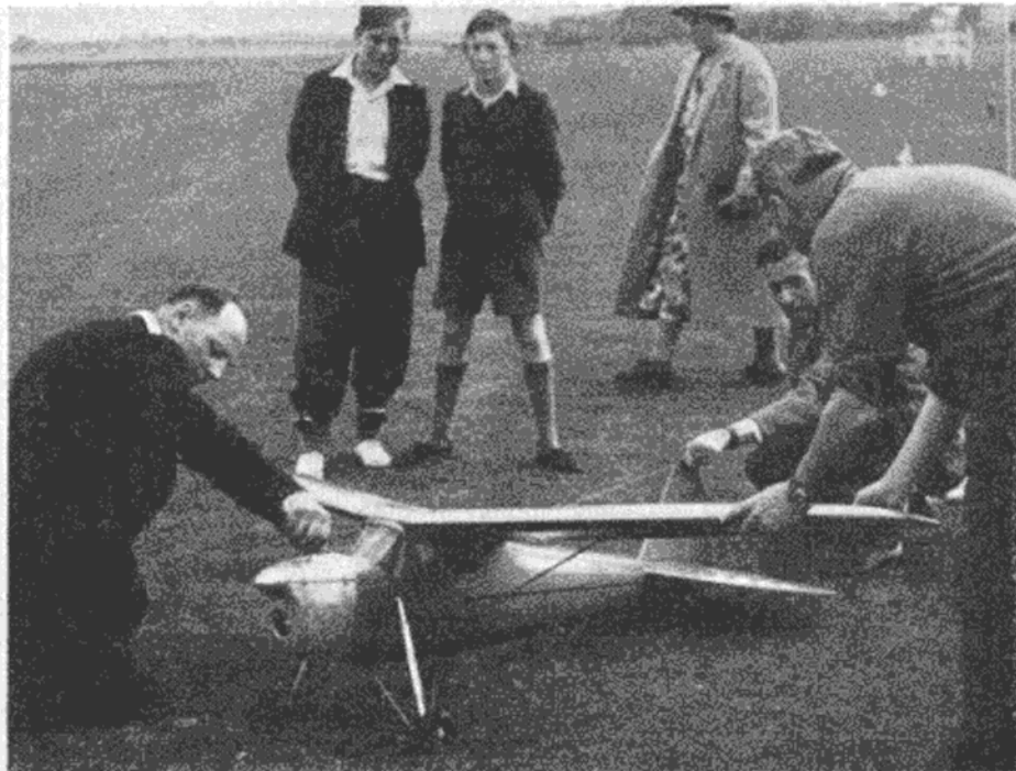
When an expert gets down to the job the result can be seen in this model of a "Mercury IV," built by Mr. Dunster of Folkestone & District M.A.C., who even designed and made the 10 c.c. glowplug engine.
