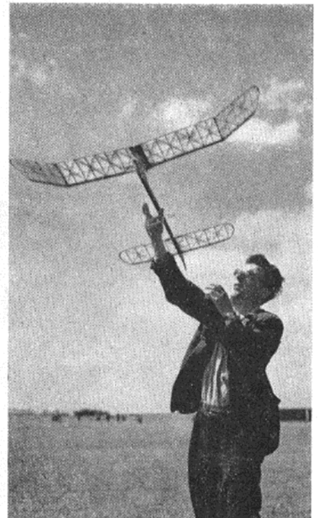
J. O'Donnell is here seen launching a Eureka, a Norman Marcus design. The geodetic bracing of the wing and tail structure is clearly visible.
