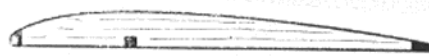
FIG. 14. UNBALANCED STRUCTURE. CENTRE OF SPANWISE BENDING RESISTANCE BELOW CENTRE OF COVERING TENSION BENDING -CAUSES BOW.
