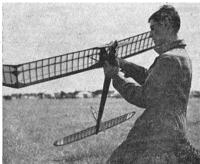
Zdenek Malina, of Czechoslovakia, adjusts his engine timer prior to making a flight in the 1958 World Power Championships at Cranfield. The model is M.V.V.S. powered and employs simple structure and wing struts. Note also the sheet underfin
