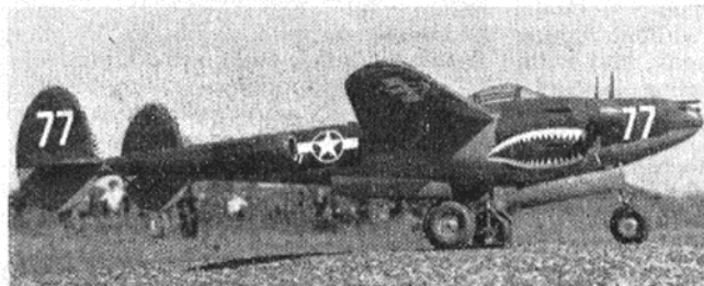
Above: prizewinning Lockheed P.38 Lightning control-liner built by P. Groos, of Haarlem, Holland. Powered by twin E.D. 2.46 diesels.
