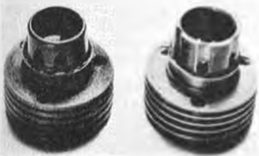
Left—differences in the porting between this and earlier models are clearly shown.
