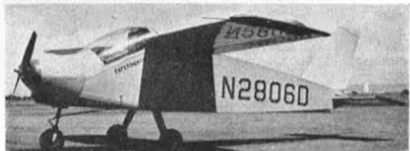
The BA-7 all metal side by side two-seater which is powered with a 75 h.p. Continental flat four engine.
