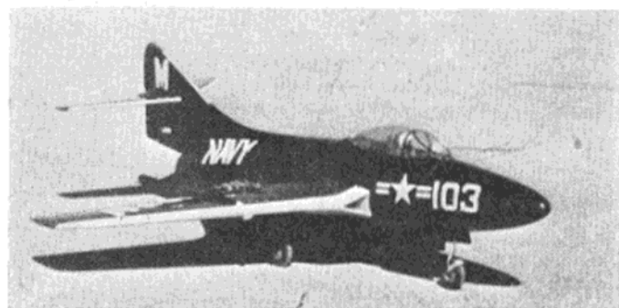
A true scale model of the Grumman Cougar jet fighter. Powered by a Dynajet pulse-jet engine of 4 lbs. static thrust, it weighs 3½-lb. and has a speed of approximately 80 mph.
