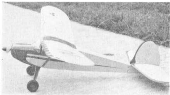
◀ Single channel R/C Nieuport 17G1 is the work of C. La Mar Kemp of Dallas, Texas (right), who is being advised on trimming techniques by Carlyle Linskie. To a scale of 2 in. to 1 ft., the model weighs 4½ lb., complete with Deltron receiver, and is powered by a Johnson "295." Colour scheme is that used by W. A. Bishop, W.W.1 fighter ace.
