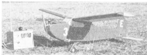
Below: Yoshiro Enya, one of the Enya engine manufacturing brothers, built this little R/C model for British E.D. radio equipment and Enya 0.06 diesel.
