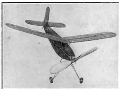
The "FIREFLY." Span 30 in., weight 2 1/2 ozs.
