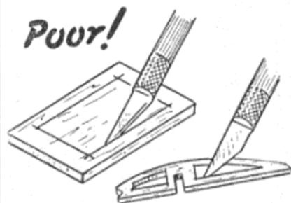
Cut-outs in ribs and formers can seriously weaken these parts, if badly made. Avoid cutting to 'square' corners with a knife or razor blade—almost certainly you will go past the line and notch the remaining wood. This means that when the cut-out portion is removed the remainder of the frame will be weak and prone to split.
