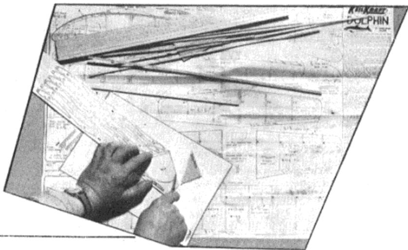
ALL model aeroplanes are built with the aid of full-size drawings or plans. These are a tremendous help. In most cases, the components of the models—fuselage, wing and tail-unit—are built directly over the plan. That is to say, the various strips of wood are pinned down over the plan and the glued joints allowed to set before each assembly is removed.
