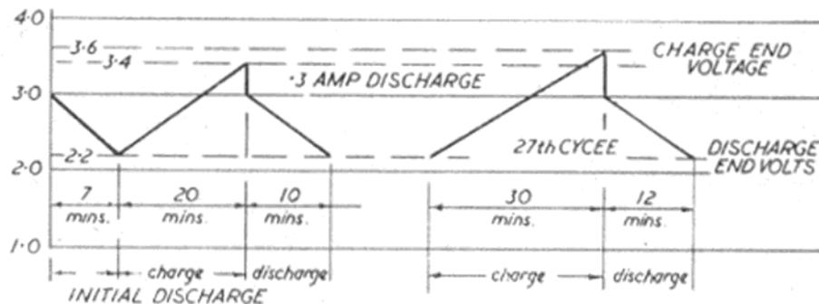
"on load" voltage has dropped to 1.1 volts per cell. It will not recharge completely dead dry batteries, nor will it give satisfactory results with batteries which have been discharged at low rates over a long period.
