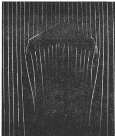
In these two photographs, airflow over two wings is shown in plan form. On the left is a typical swept wing with raked tips. The angle of attack is quite moderate and the special points of interest are the twisting of the airflow past the tips (actually the air is trying to roll up into a vortex trailing from each tip) and the deformation of the airflow over the wing itself. The position of individual filaments reaching the leading edge and leaving the trailing
