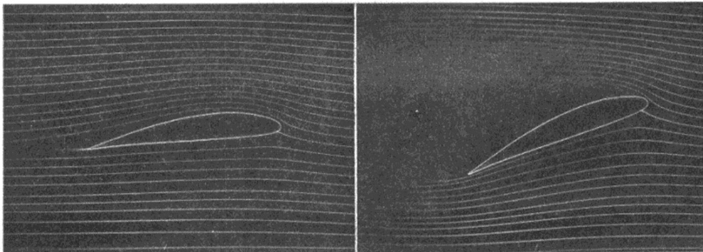
The following sequence of photographs, which are reproduced by kind permission of the Collins Radio Company of America, show various wing sections and plan shapes under visual airflow test in their wind tunnel.
