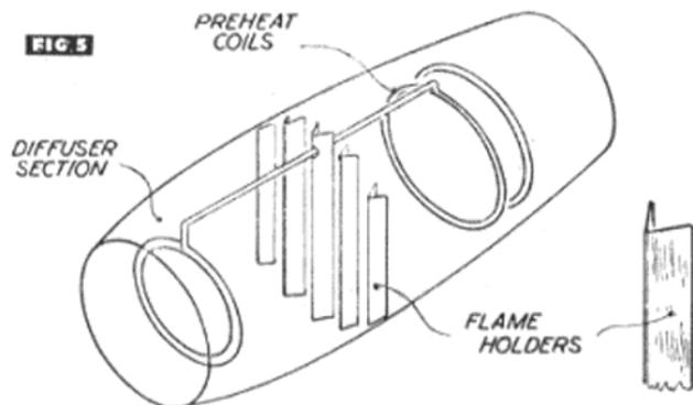
combustion chamber, a series of these strips giving a sort of venetian blind effect with vertical slots between them. Spacing and positioning for optimum effect would have to be determined by cut-and-try methods.
