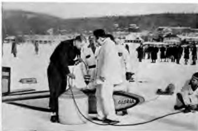
Above.—The tanks were placed on the c.g. so that balance would not be upset as the propellant was consumed. Illustration shows the charging of the 'plane with liquid oxygen.
