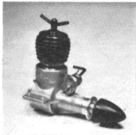
The Taifun Hobby of 0.99 c.c. A well-made unit with pleasant handling characteristics, this model supersedes the Taifun Junior of the same capacity.
