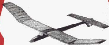
51" span contest glider with an outstanding performance 15/9
