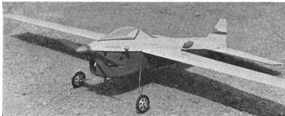
"Polaris 1960" latest team-racer by Czech champion Milan Drazek. Powered by works-modified Oliver driving 6.9 x 8.7 in. prop. High a.r. 39 in. span wing. Speed 93-96 m.p.h. A probable entry in the forthcoming World Championships.
