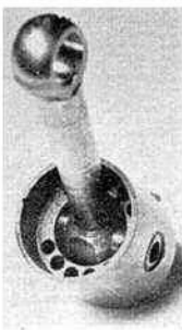
Below: left, the modified crankshaft with enlarged port and chamfered web; right, lightening holes drilled in piston.
