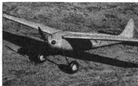
Typical of the early radio controlled models is this 12 ft. span job by Earl Vivell, which weighed 26 lb. Using selective single channel control working rudder and elevators, it flew well with a 1/2 h.p. motor in America in 1940.
