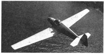
R.F.o1 monoplane illustrated above. At first glance it looks a fairly conventional single-seat cabin monoplane, but those long-span (36 ft. 9 in.) wings enable it to double as both a sporting aeroplane and a training sailplane, with power off.
