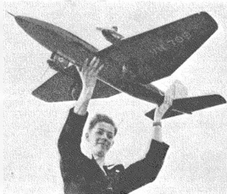
A. W. Major and his twin Frog "500" powered E.E. Canberra . This model was scaled up from a 1/72 scale kit drawing.
