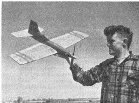
A modern semi-scale control-line stunt model. This machine, which was built from a kit, is powered by a 3.5 c.c. engine.
