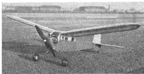
Large prop on this E.D. 3.46 powered "Junior 60" eliminates risk of a power-on crash in the event of radio failure.
