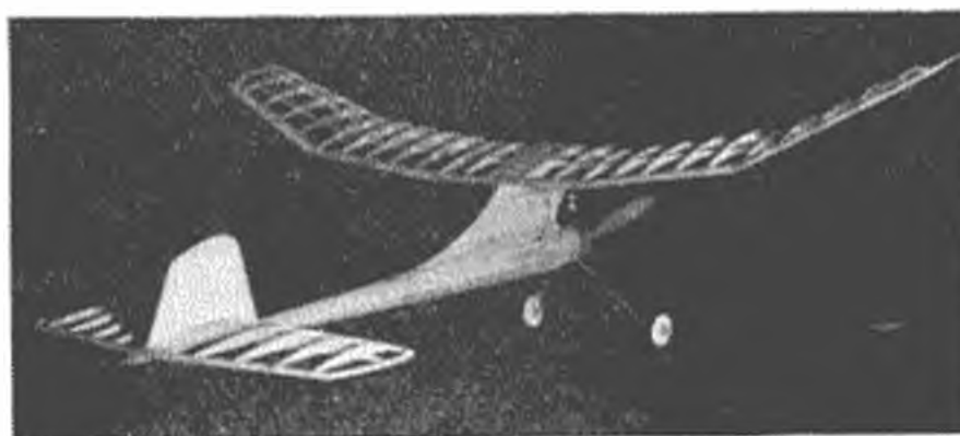
Another typical power-duration model before covering. One of the most popular contest types, these models are capable of very high rates of climb.
