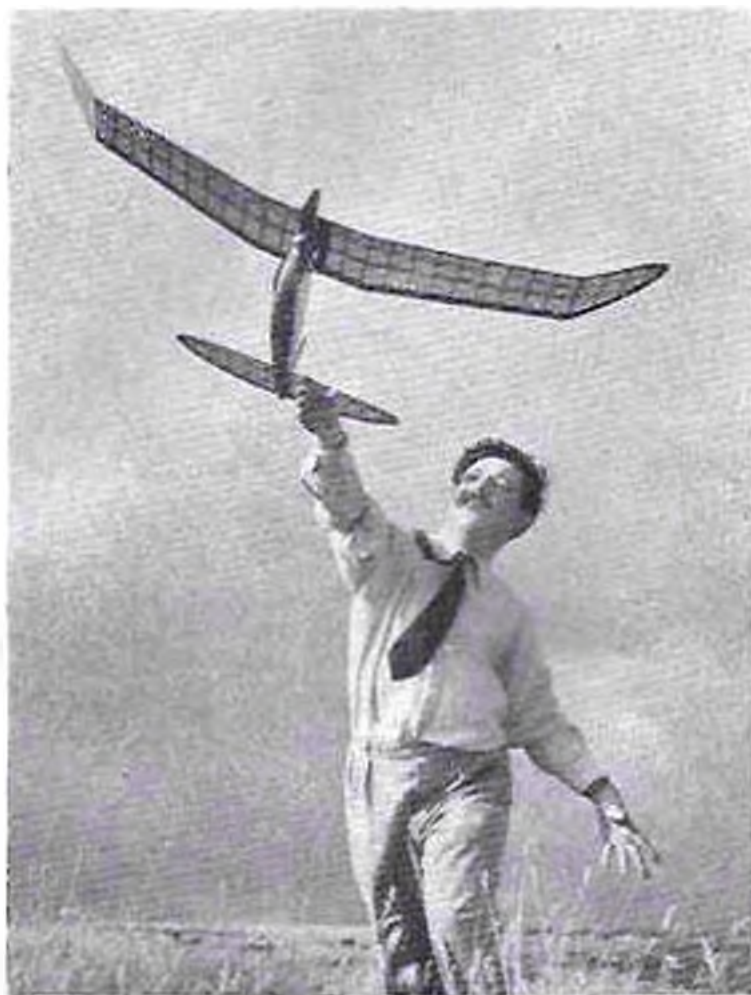
Bill Blake test gliding his American designed "Zeck." Span is 50 in., and wing area 385 sq. in. Bill is well known for his many successful F.F scale designs.
