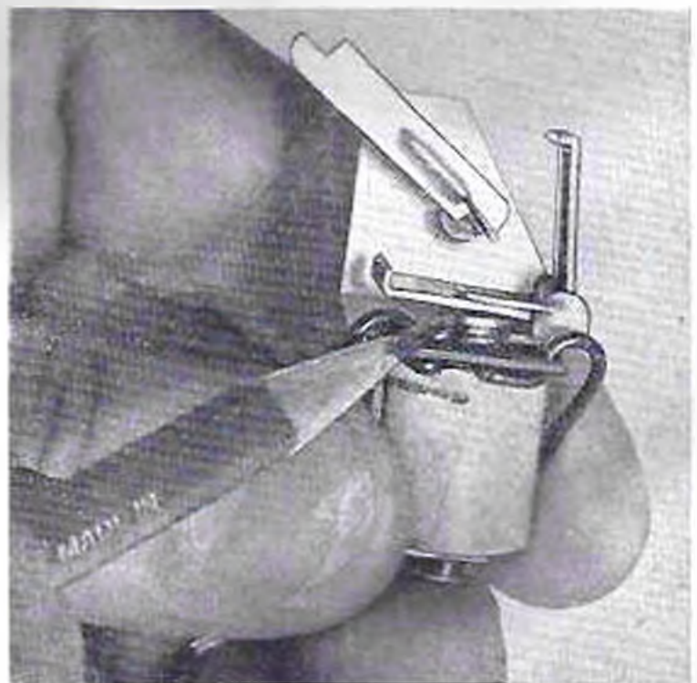
A small piece of tissue cemented to the armature or magnet pole will prevent the actuator from sticking.
