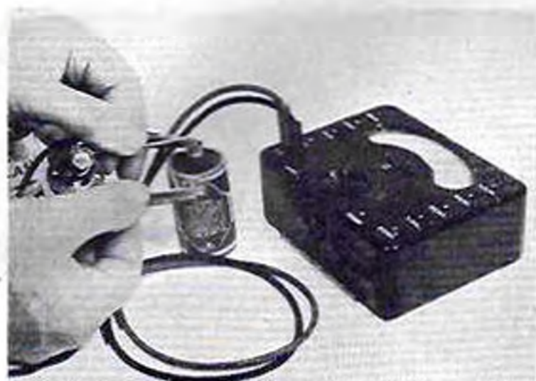
A simple load test made with a 3.5 V bulb and holder.
