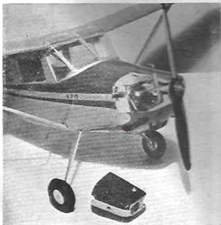
The "Cessna 170" with cowling removed. Note dual undercarriage legs.
