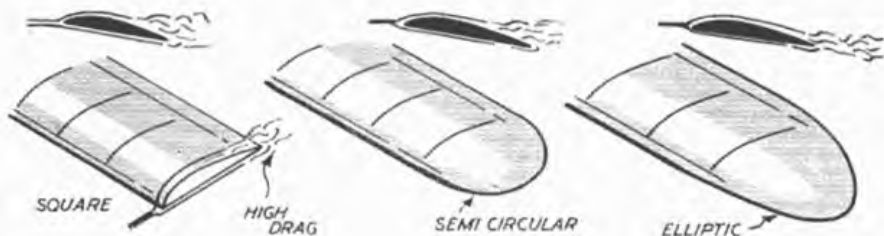
HIGH DRAG FROM SQUARE TIPS AT HIGH ANGLES OF ATTACK
