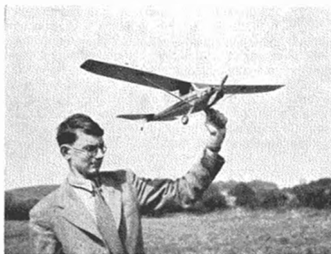
40-in. span Luscombe "Silvaire" built by John Vaughan from a K-K kit. Model flies excellently and is powered by an Allbon "Dart" diesel.
