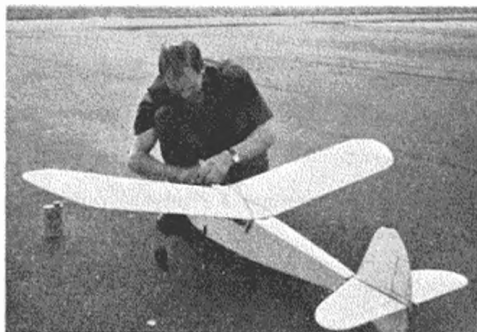
C. G. Sallis of Littleport, Cambridge, starts his R.C. "Junior 60." Engine is on E.D. 2.46. Receiver: E.C.C. 951A hardvalve.
