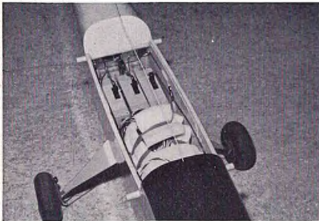
Fuselage view showing equipment installation — receiver (Digimite) is wrapped in foam. Antenna has since been put back inside. This is the wire running near the top along the right side.
