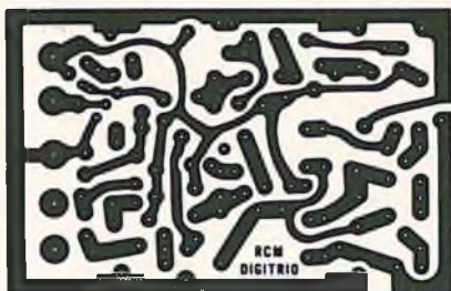
Decoder PC board shown three times full size. Actual size PC board shown at left. Either can be used for photographically reproducing the circuit board.
