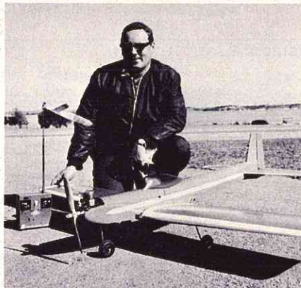
Chuck Cunningham with his Mustang red "Ply-Fli" a modified Sun Fli with one piece "folded" plywood fuselage and cardboard covered foam wings.
