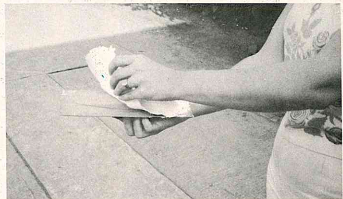
Peeling mold from plug. Next, trim with scissors.
