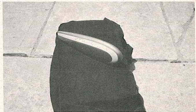
Finished wheel pant made from 3 layers of fibreglass cloth.
