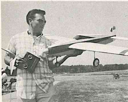
W. Jersey Radio Flyer, Jim Martin, and "Eye Ball". 6½ lb. ship had Webra B/H 60, Micro-Avionics radio. Lateral area helped on slow rolls, knife edge. Great side-slip ability.
