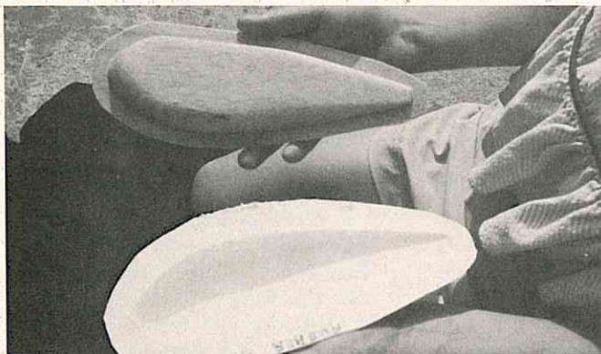
Photo of wheel pant half and silicone mold.
