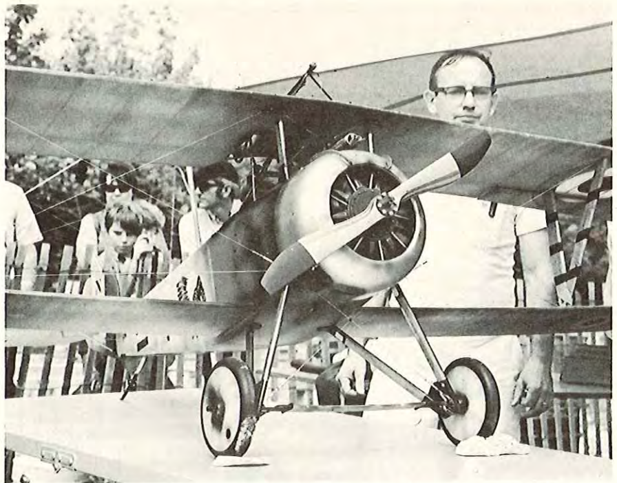
Harold Penny's 3" scale Nieuport 17 used O & R Compact engine, weighed 12 lbs., 11 oz.
