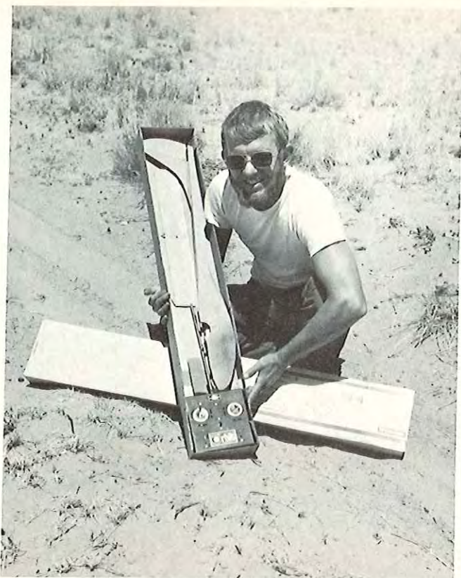
"This is the way we stow our planes, stow our planes . . ." Clod Nine nestles in foam wing box. Transmitter is padded with foam. Wings join by wire-and-tube method.
