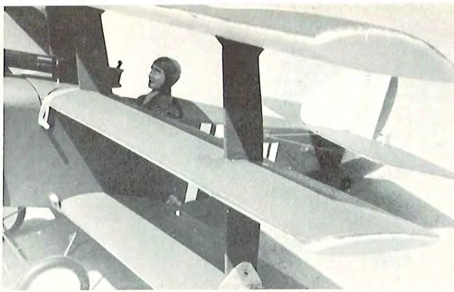
ABOVE: Detail view of outer wing struts. Plywood units are epoxied into top wings and bolted to lower foam wing panels. BELOW: 'Seuenstrand' fishing leader cable and ply horns add to realism but standard pushrods can be used.
